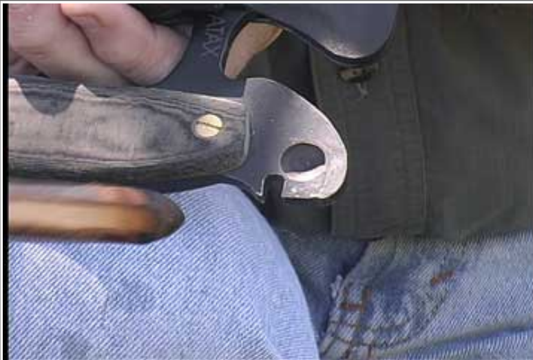
One of the unique features of the tool is the divot used as both a fire bow bearing and a leveler for direction finding.
