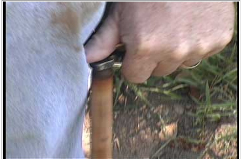
Pressure is put onto the top of the drill through the tool...
