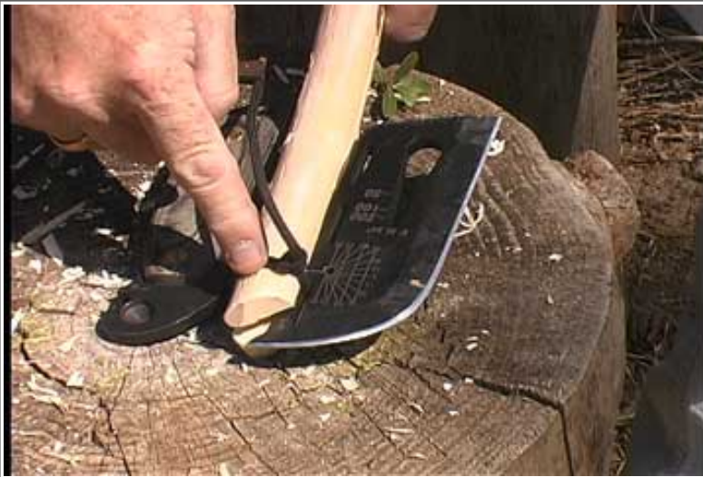
One of the prime uses for the tool is as an AX. That's what put the AX in ATAX. Here we show how to bind the tool to a split stick for use as a chopper.
