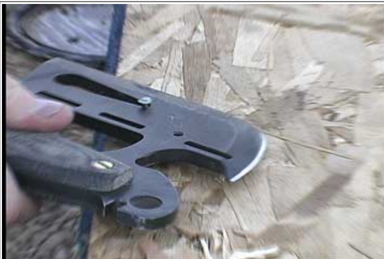
Here you can see the head of the nail in the rangefinder/wrench slot.
