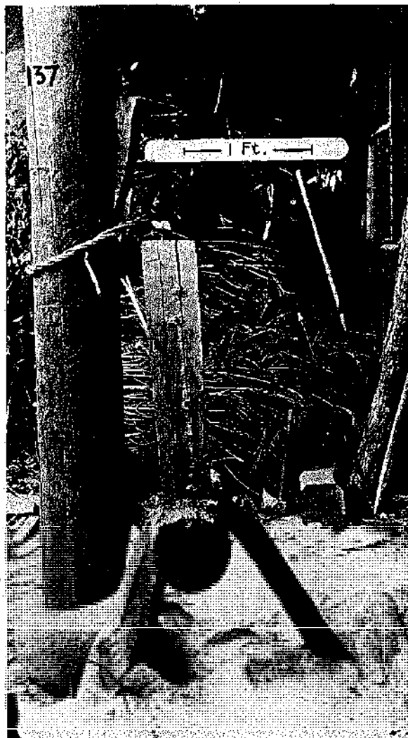
FIG. 532. COOPER'S CLAMP FOR SAWING OUT TUB STAVES.
