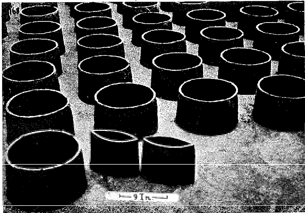
FIG. 411. CLAY CYLINDERS ON THE DRYING FLOOR. ONE IS BROKEN UP INTO ROOFING TILES.
