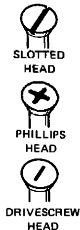
Fig. 12-3 Three types of screw heads.
