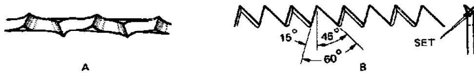
Fig. 7-25 How teeth should appear when completed.
