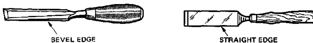
Fig. 9-10 Wood chisel blade shapes.
