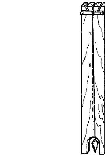
Fig. 5-14 Using a plumb rule to align the plumb line with the pencil line.
