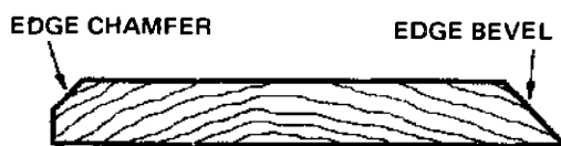
Fig. 8-38 Comparing a chamfer to a bevel.
