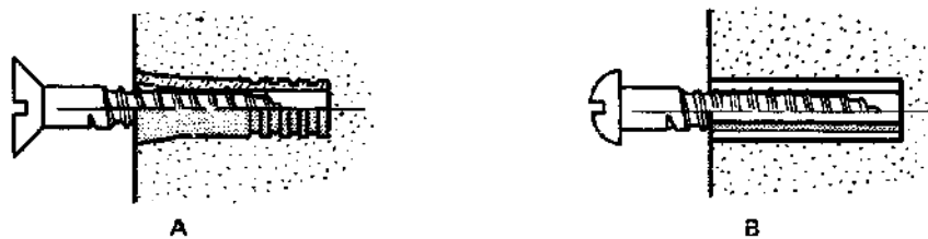
Fig. 12-27 (A) Application of a lead shield (B) Application of a plastic expansion plug
