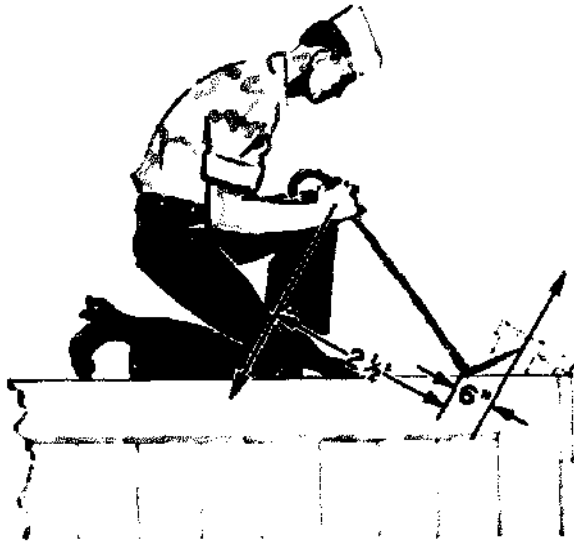
Figure 1-12.—Using a wrecking bar.
