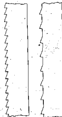
The standard blade pattern is shown on the left. The other is a skip-tooth or "buttness" design.
