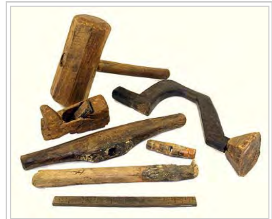
Carpentry tools recovered from the wreck of a 16th-century sailing ship, the Mary Rose. From the top, a mallet, brace, plane, handle of a T-auger, handle of a gimlet, possible handle of a hammer, and rule.
