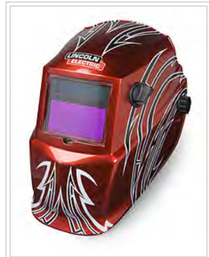
Auto darkening welding hood with 90×110 mm cartridge and 3.78×1.85 in viewing area
