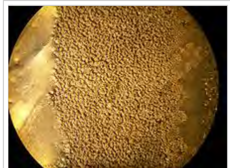
Closeup view of an aluminum TIG weld AC etch zone
