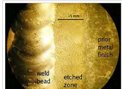
A TIG weld showing an accentuated AC etched zone
