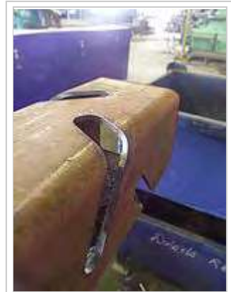
Metal cutting by plasma arc.
