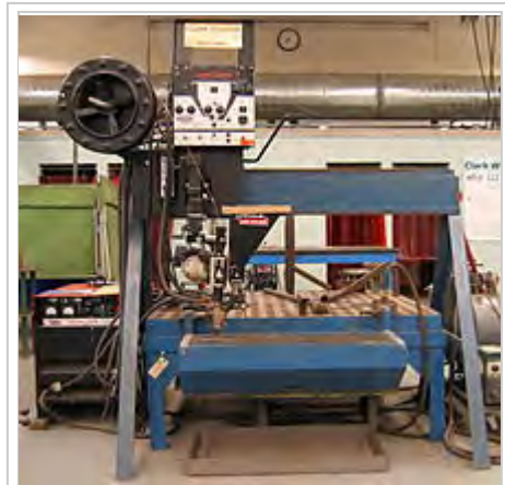
A submerged arc welder used for training
