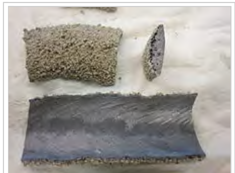
Pieces of slag from Submerged arc welding
