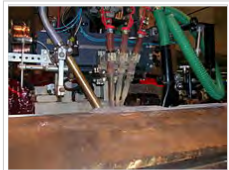
Submerged arc welding. The welding head moves from right to left. The flux powder is supplied by the hopper on the left hand side, then follow three filler wire guns and finally a vacuum cleaner.
