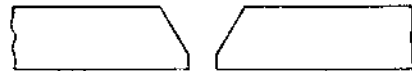
\frac{1}{4} " to \frac{3}{4} " 60° single "Vee" - \frac{1}{16} " to \frac{1}{8} " gap Root face \frac{1}{32} "
