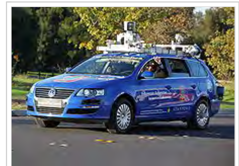
A robotic Volkswagen Passat shown at Stanford University is a driverless car
