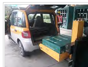
The battery swap process on a Zotye M300 EV.
