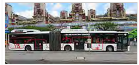
Battery electric bus powered with lithium-ion batteries
