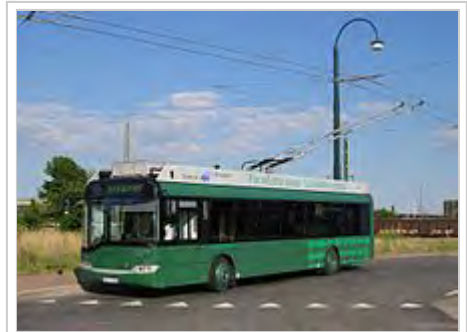
A trolleybus uses two overhead wires to provide electric current supply and return to the power source
