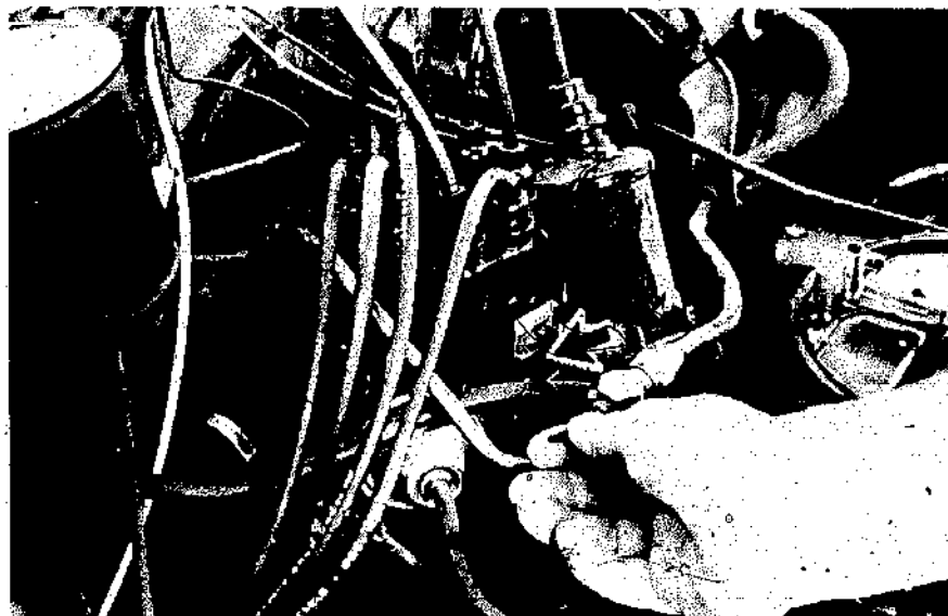
Adjusting access window on GM distributor.
