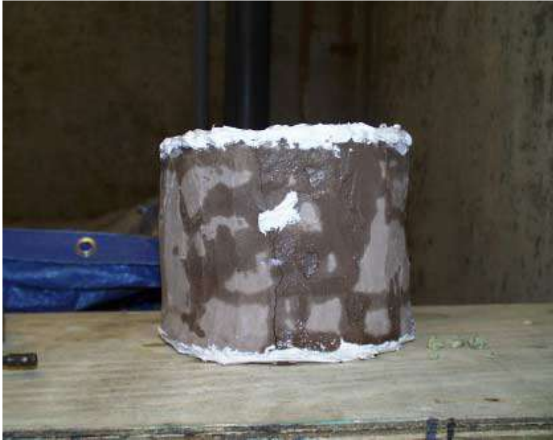
Figure 23: A sample with end leakage
