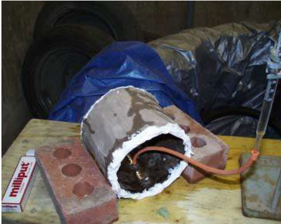
Figure 21: set up of the rig showing pipe connecting to channel and pipette
