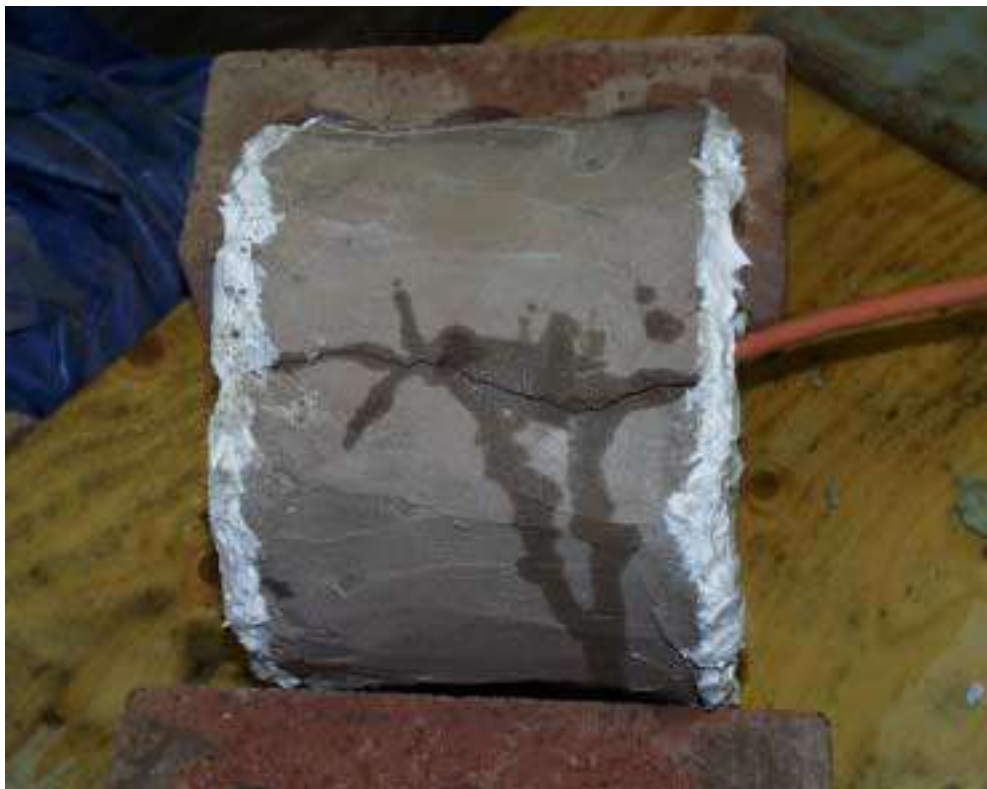
Figure 22: Leakage through a crack
