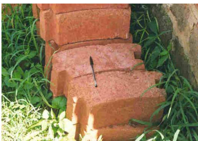
(Figure 6.3 – Curved blocks after curing)
