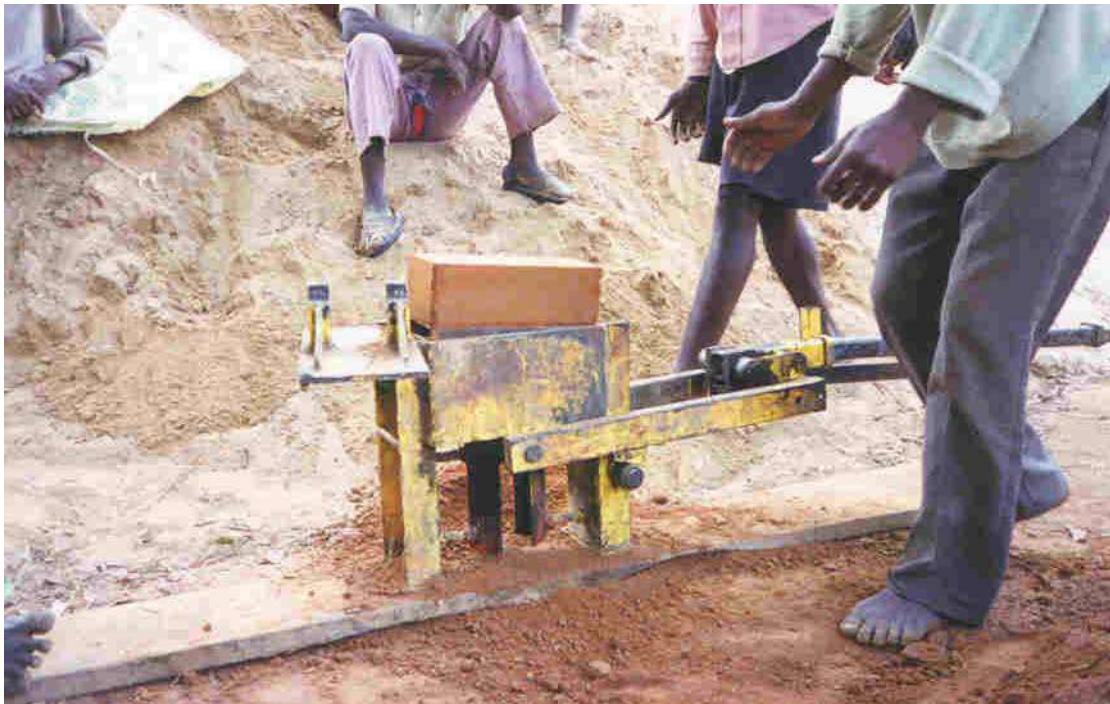
Figure 2.3 A CinvaRam press being used to produce stabilised soil blocks in Africa
