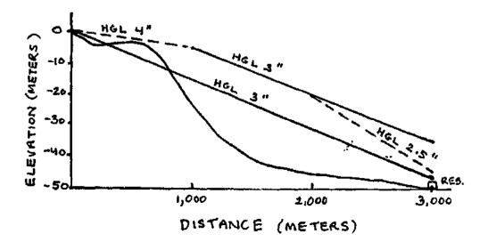
P.17. The figure below contains a ground profile from a water source to a reservoir located at a mosque 2,000 meters from the source.
