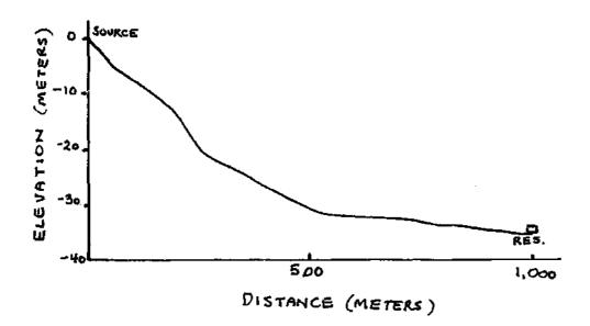
S.13. The available head from the source to the reservoir is approximately 35 meters. Using the water flow calculator the following values are obtained for a flow of 2 1/s using GI pipe:
