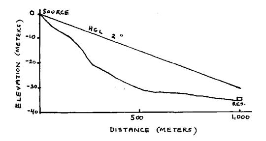
P.14. Given the ground profile and design flow in the figure below choose appropriate GI pipe. Plot the HGL for the pipe selected.
