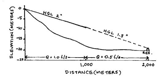
P.15. Given the gound profile in the figure below plot the HGL for a design flow of 4 1/s using 3 inch GI pipe.
