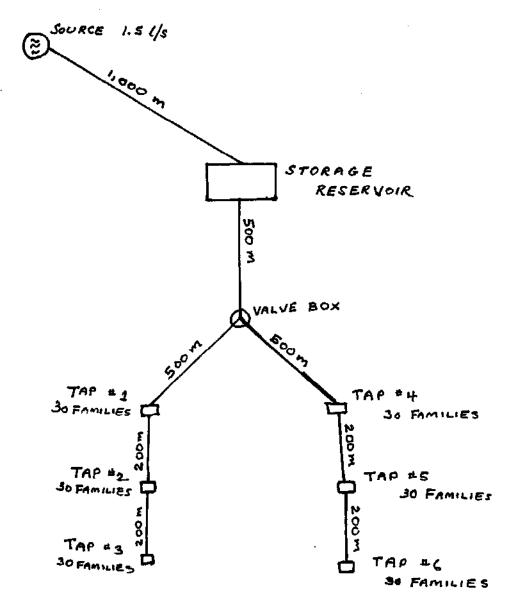
P.21.1. In this system a storage reservoir will be constructed 500 meters from the village. Recommend an appropriate volume for the storage reservoir. How was this volume calculated? Suggest approximate dimensions for the reservoir?
