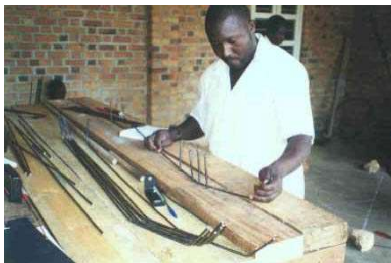
Figure 2 – Workbench fitted with bending jig – the angles for the spokes are marked on the jig to make the process quicker and easier
