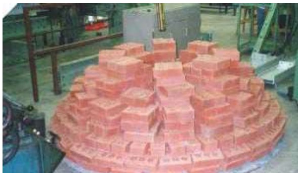
Figure 21 - Tank cover loaded to 1000kg
