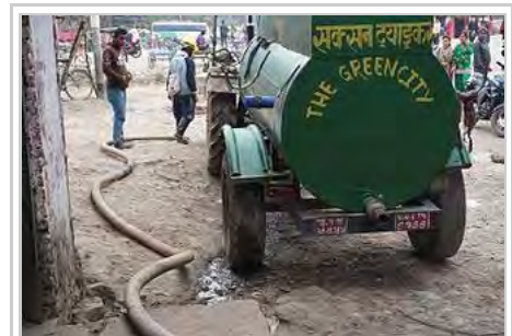
Desludging truck (vacuum truck) in action in Nepal
