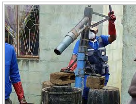
The "Gulper", a device for manual pumping of fecal sludge from pits used in eThekwin (Durban), South Africa.
