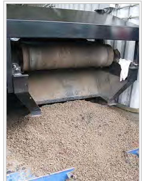
Sludge pellets after processing (including heating, drying and pelletizing) in a LaDePa process, eThekweni Municipality (South Africa)
