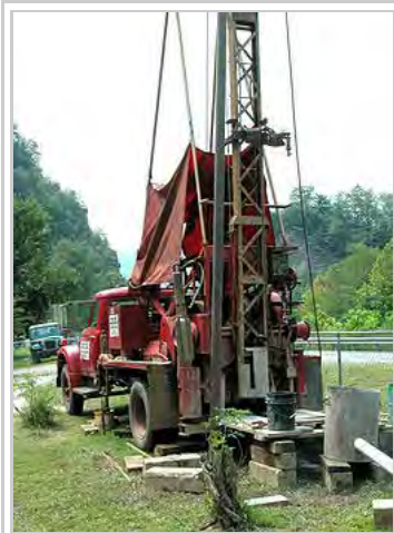
Cable tool water well drilling rig in Kimball, West Virginia, USA.
