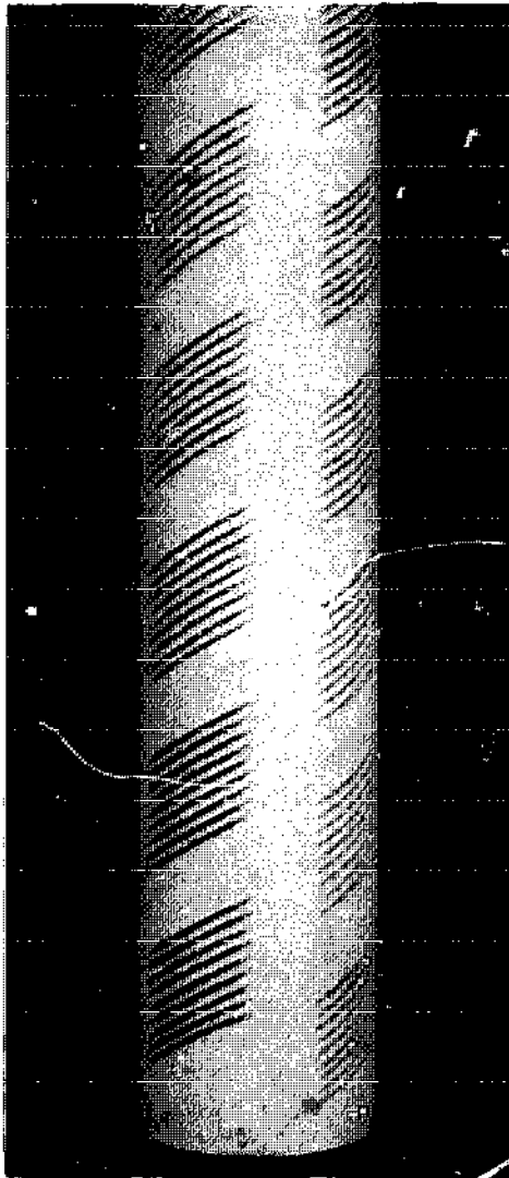
Fig. 4.6 SLOTTED PLASTIC PIPE.
