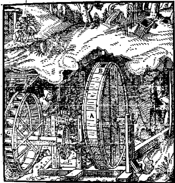
Fig 2.51 (a) Draining a mine in the sixteenth century, with an over-shot waterwheel driving pumps to lift the water in two stages. (b) Sixteenth century mine ventilation using a fan driven by a waterwheel From De Re Metallica by Georgius Agricola, 1556
