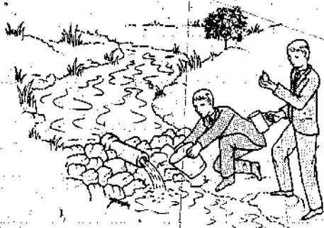
Fig 2.12. Measuring flow by damming and inserting a pipe
