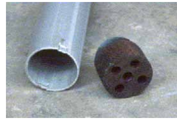
Riser pipe and valve
