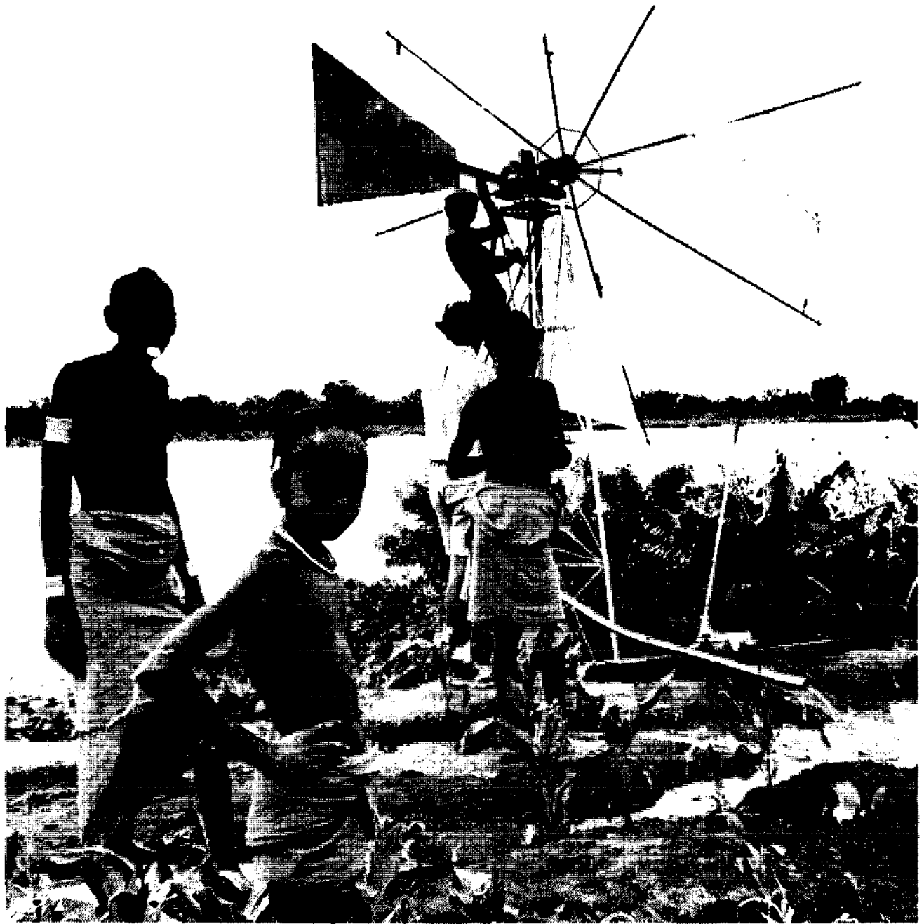
A typical "Polomo" Cretan-type windmill delivering water to a Geleb plot – the owner is on the left. Only four sails are deployed in this picture.
