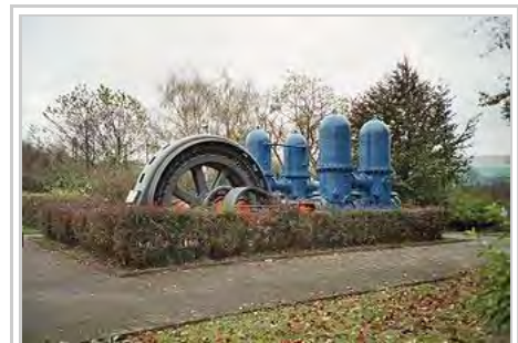
A large, electrically driven pump (electropump) for waterworks near the Hengsteysee, Germany
