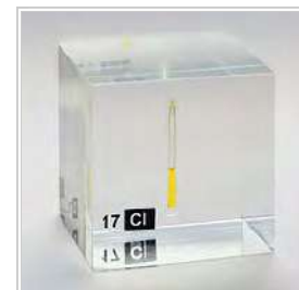
Chlorine, liquefied under a pressure of 7.4 bar at room temperature, displayed in a quartz ampule embedded in acrylic glass.
