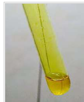
Yellow chlorine dioxide ( \text{ClO}_2 ) gas above a yellow chlorine dioxide solution. Solutions of pure chlorine dioxide are dark green: this solution is yellow due to impurities produced from its photodecomposition.
