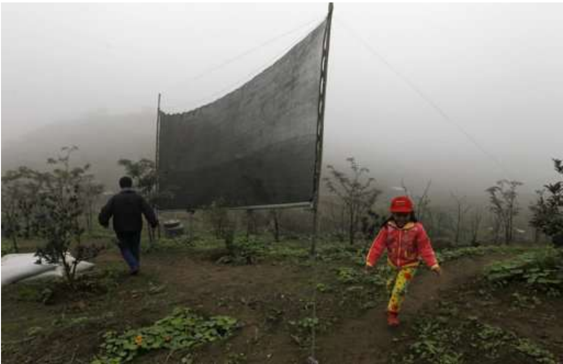
The fog that settles every winter morning on Lima now serves to irrigate crops in the nearby desert hills thanks to a "fog-catchers", a simple and cheap system that collects and condenses fog to produce between five and 15 liters of water per day.
