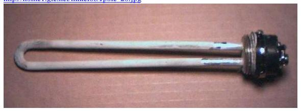
Warning: Running the eclectic heat element without water only lasts for a mater of seconds before the heater element burns out. It makes a popping nosed which is not all that laud. Changing out the heater element is the only thing that can be done to fix this. Cost is about \$8 at Home Depot. You may want to stock up on as many spares as you can afford.
