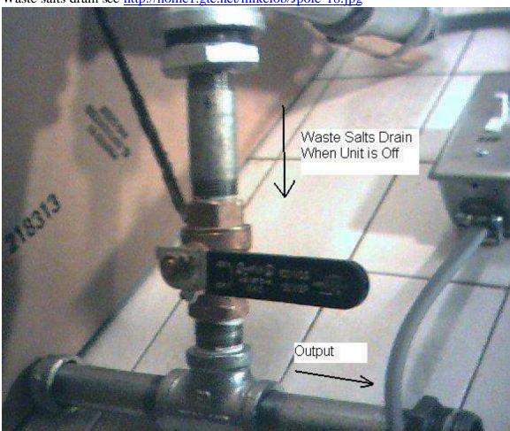
This upside down "T" has two purposes. It helps hold the unit up and it allows salts to be drain off when the unit is turned off. Neither one are essential to operation. The unit designed for open fire use has a clean out plug at this point. The salts tend to deposit on the walls of the boiler tube with time. Frequency of cleaning will depend on the hardness of the water source.
