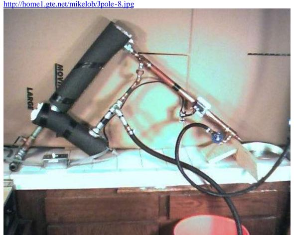
Use insulation like shown in the picture to keep the heat in. This adds about 5 percent to the efficiency of the unit.
