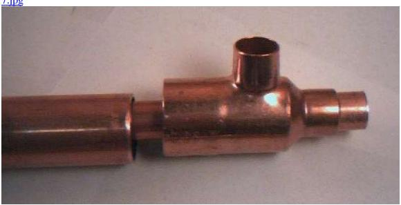
The heat exchanger is made up of two pipes one on the inside of the other. Steam flows down the center .5 inch inner pipe being cooled by water held around this by a 1 inch outer pipe. The end caps are 1" x .5" x .5" copper "T" fittings with the ridge filed off on the inside so the .5 inch pipe slips completely through it. The 1 inch pipe is 20 inches long and the .5 inch is 25 inches long. This or longer will work fine.
