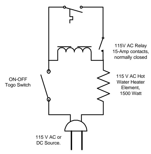
If the cooling flow stops then the temperature switch will turn off the current flow to the heater element. If the water flow stops totally then about 40 sec latter the 150 degree F
