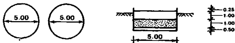
Figure 4.2. Dimensioning of slow sand filters
