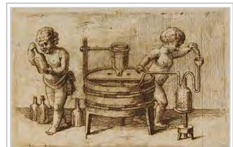
Drawing of an apparatus for studying the chemical analysis of mineral waters in a book from 1799.
