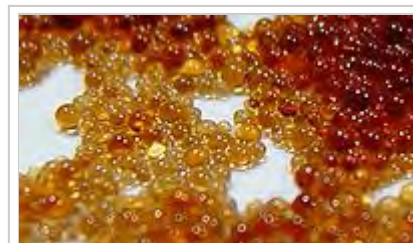
Ion exchange resins, in the form of beads, are a functional component of domestic water softening units.
