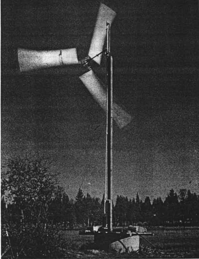
The sail-wing machine in action, pumping water from an artesian well close to ground level.
