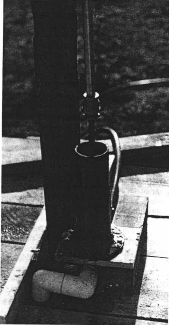
Sucker rod and water pump used with the sail-wing. The sucker rod pushes down on leather pump seals, driving a pulsing stream of water into the plastic pipe at rear.
