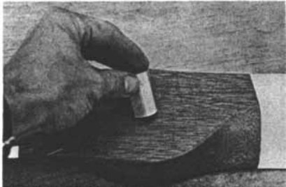
Fig. 11-15. The bushing should fit snugly in the center hole.
