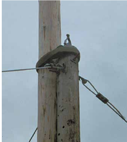
Below: Top of the gin pole showing nylon strap, guy attachment, and fairlead pulley.
