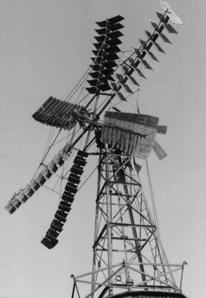
Wind machine for mechanical power, for farm or small factory use. Photographed in March 1994.
