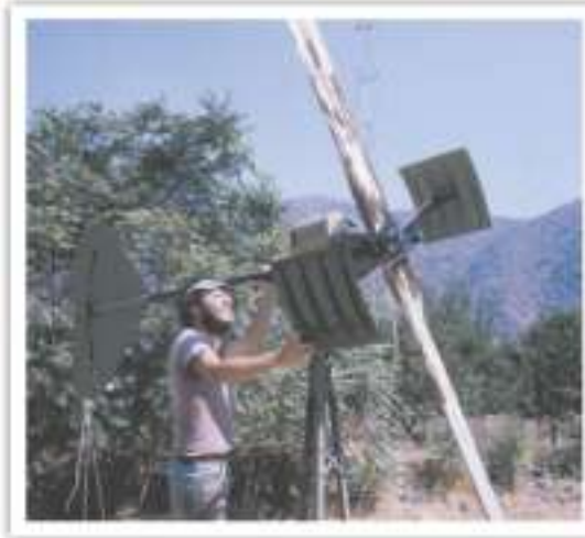
(Left) A damaged Wincharger sits atop a tower in Wyoming. In a stiff wind, Michael Hackleman hoists it clear (inset) and lowers it. This is the machine Craig Worthley would restore.
