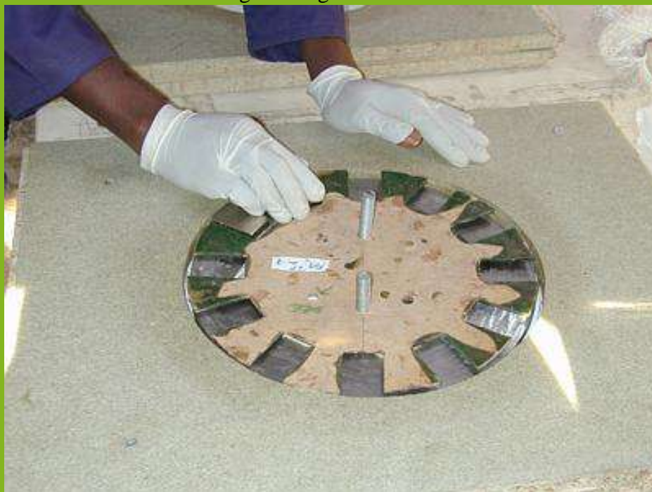
Fitting the magnets on the disk
