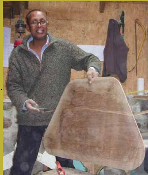
Cutting out the plywood tail vane.
