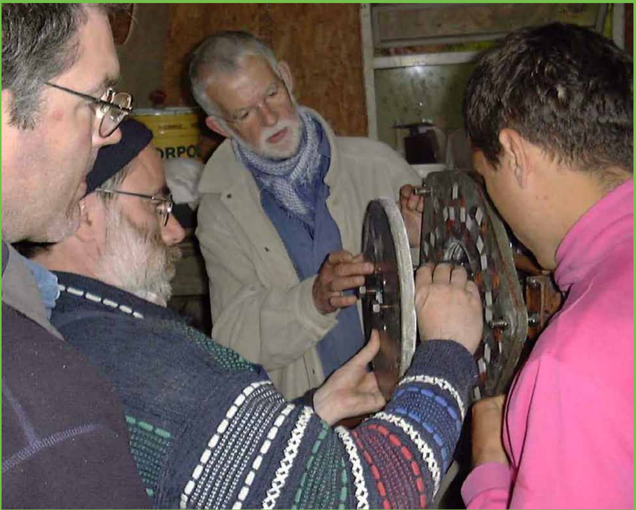
Pic 23: The jacking screws work wonder. Actually, the attraction of the Neodymium magnets is so strong it would be impossible to control the assembly process without them.
