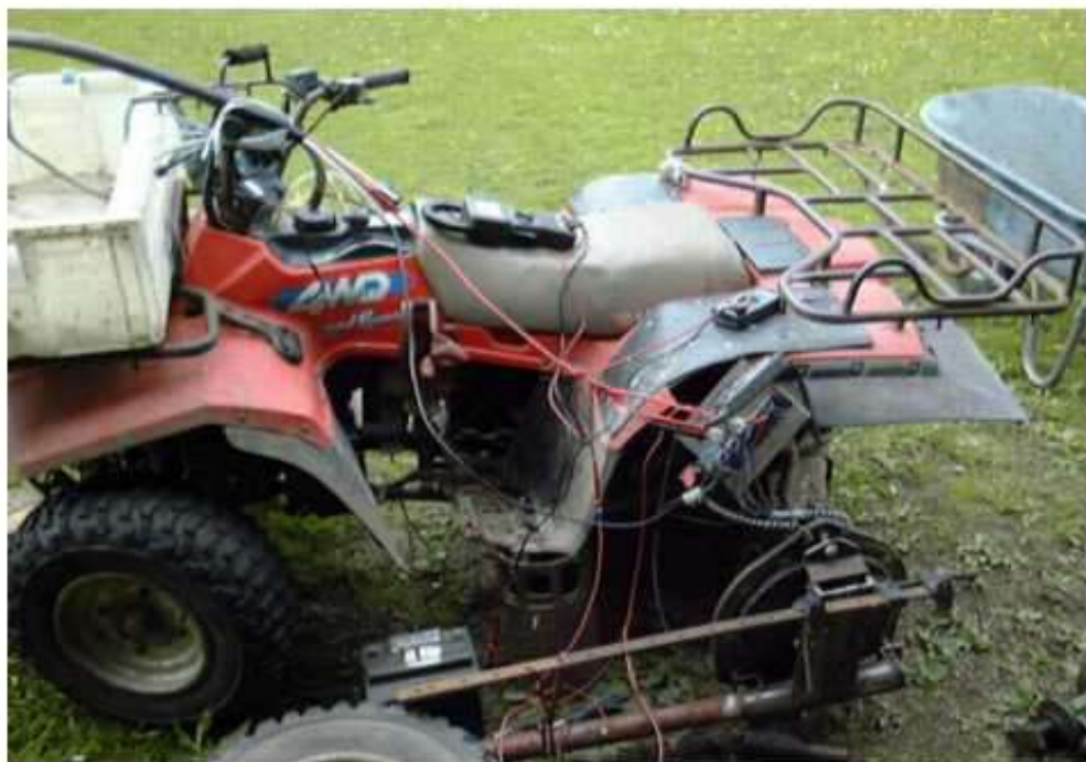
Testing the alternator on the rear wheel drive of our quad bike.
