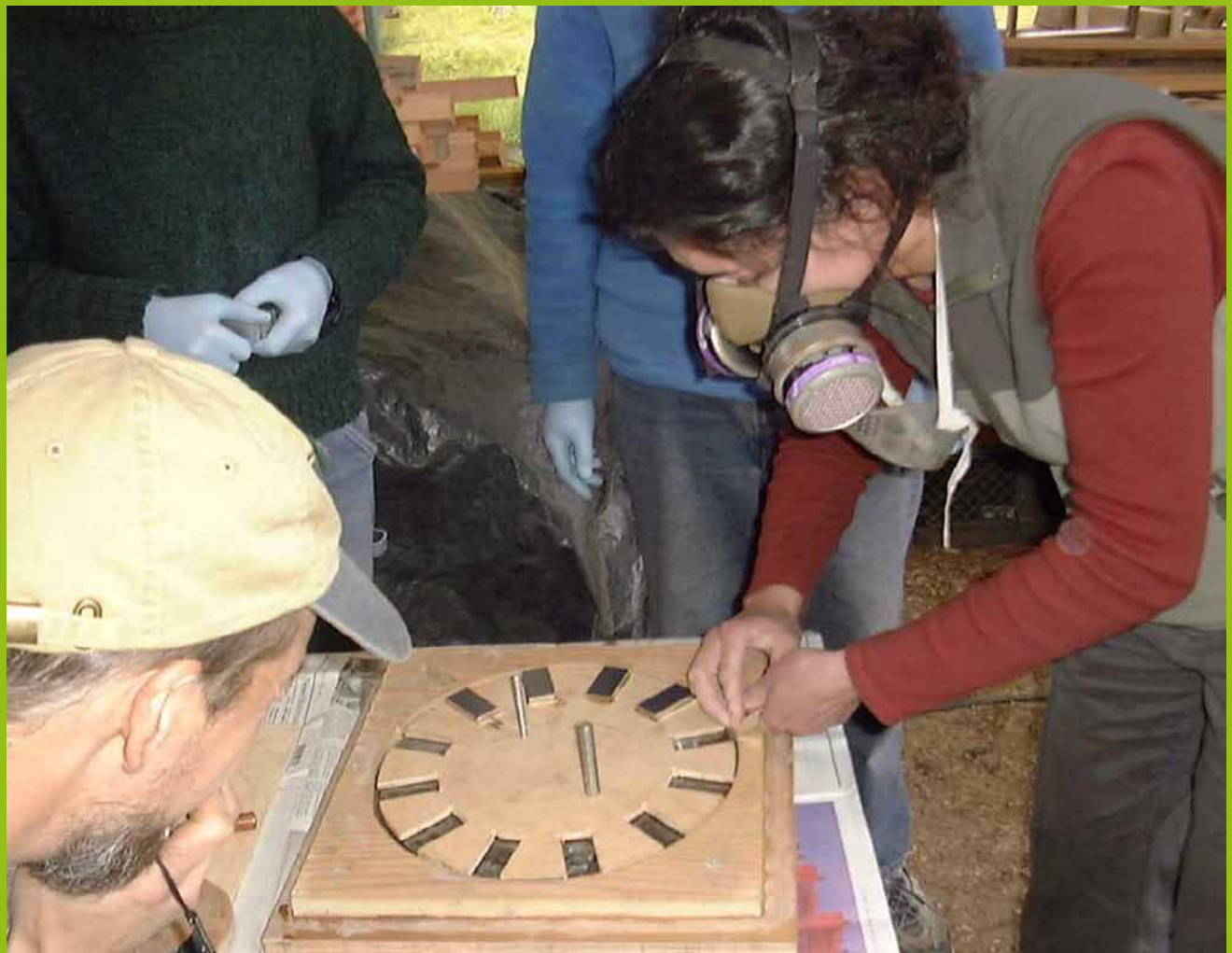
Adding magnets. The respirator is to protect against styrene monomer solvent fumes from the polyester resin.
