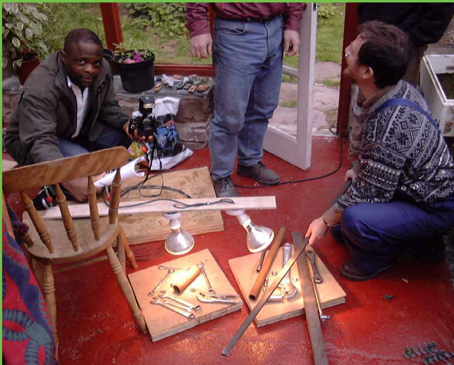
Pic 16: The reusable stator moulds have been opened, it turned out just perfect. After pouring the resin it is important to vibrate the moulds so air bubbles can rise to the top. Neodymium magnets will deteriorate when exposed to harsh environments, the resin not only prevents the magnets from flying away but also from aging. (Neodymium magnets suffer deterioration if water manages to penetrate the protective coating. Embedding them in resin seems a good idea. - Hugh)
