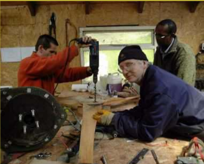
Assembling and balancing the rotor blades.
