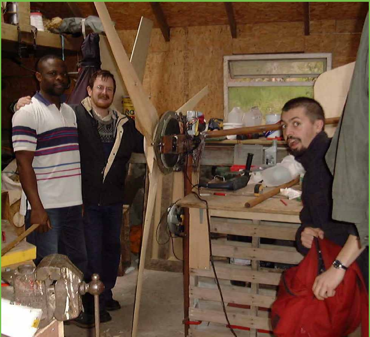
Pic 29: Oops, a fuse blew. It is and was good advice to always use fuses with battery circuits, discharging currents can be huge. Julius Tangka flipped the polarity of the alternator wires and everything was OK then - after we used a new fuse.
