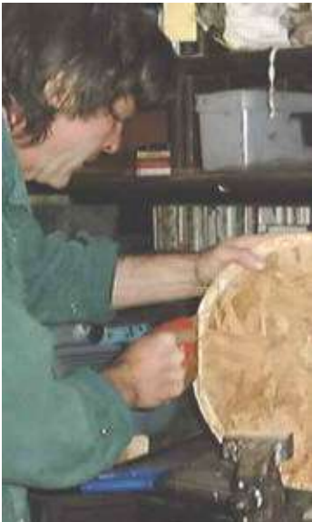
Sawing flat faces on the inner mould
