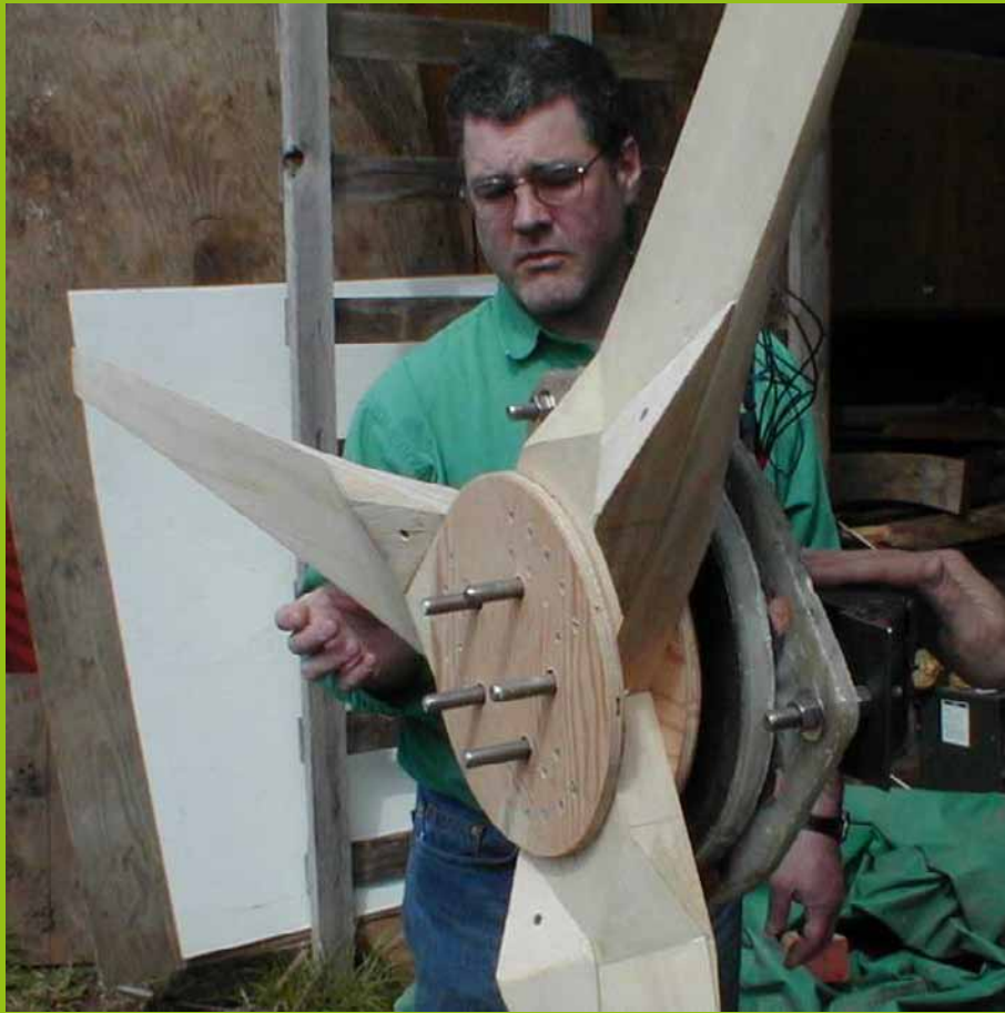
The blades on the alternator (8' diameter machine).
