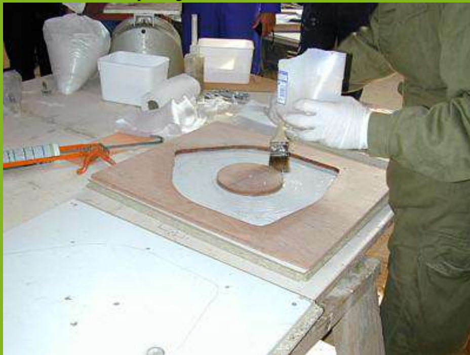
putting resin in the statr mould
