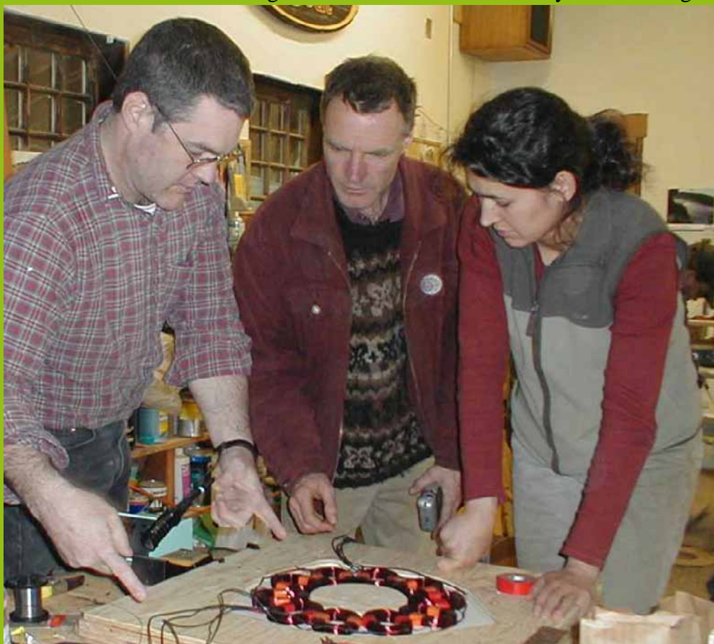
Brian Faley was in charge of the resin cast components. The electrical and magnetic parts of the alternator were cast in polyester (fibreglass resin).
