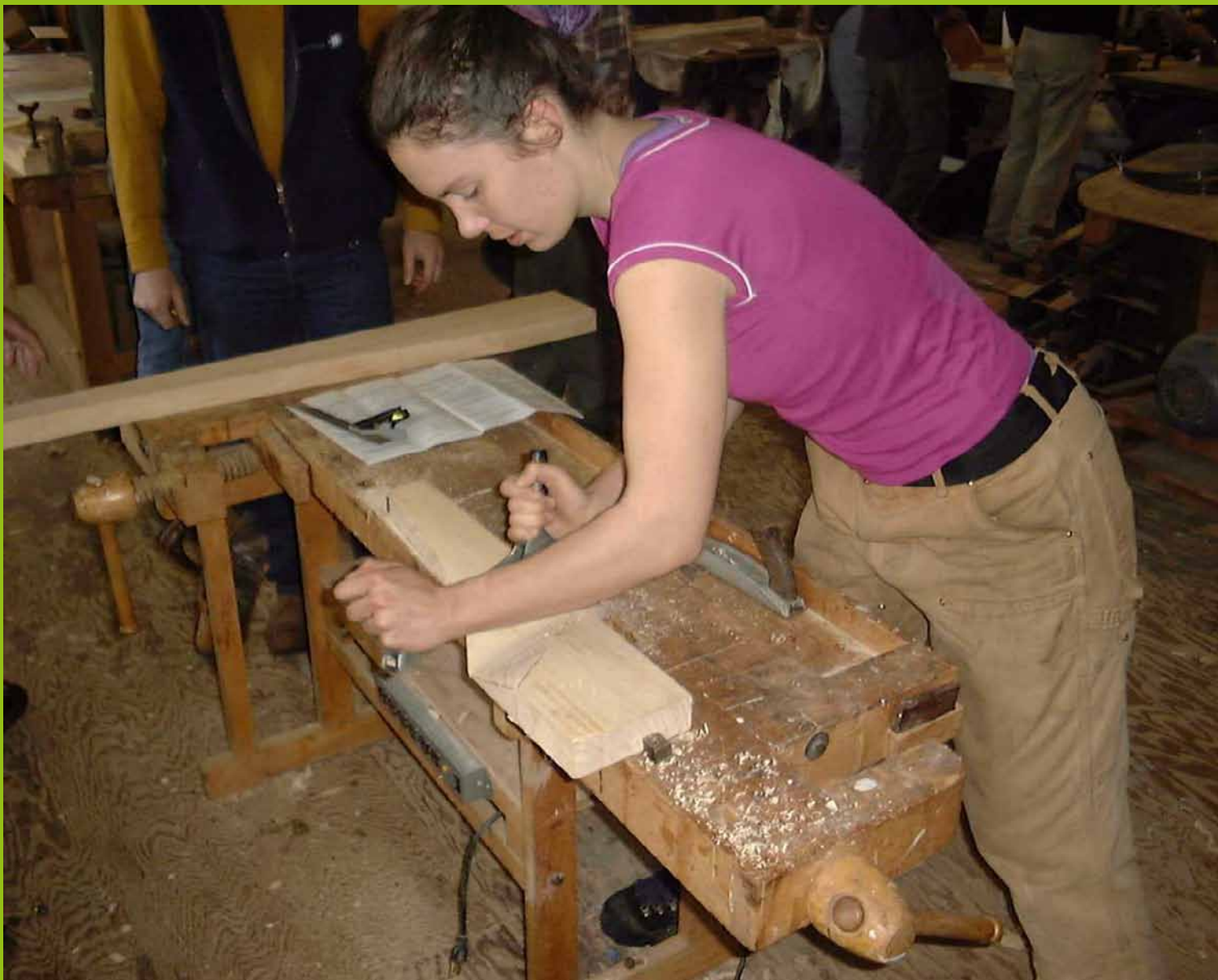
Ellyn using one of many approaches to cutting out the 'scoop'. I prefer to use the draw knife for this job.
