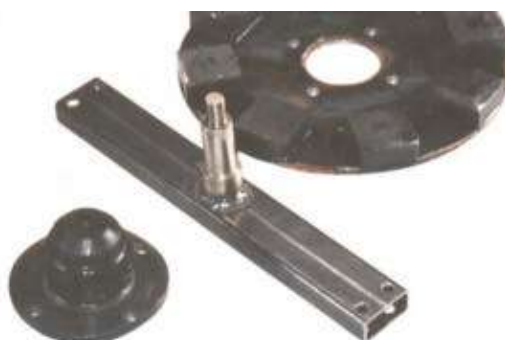
Spine, shaft, hub and magnet rotor
