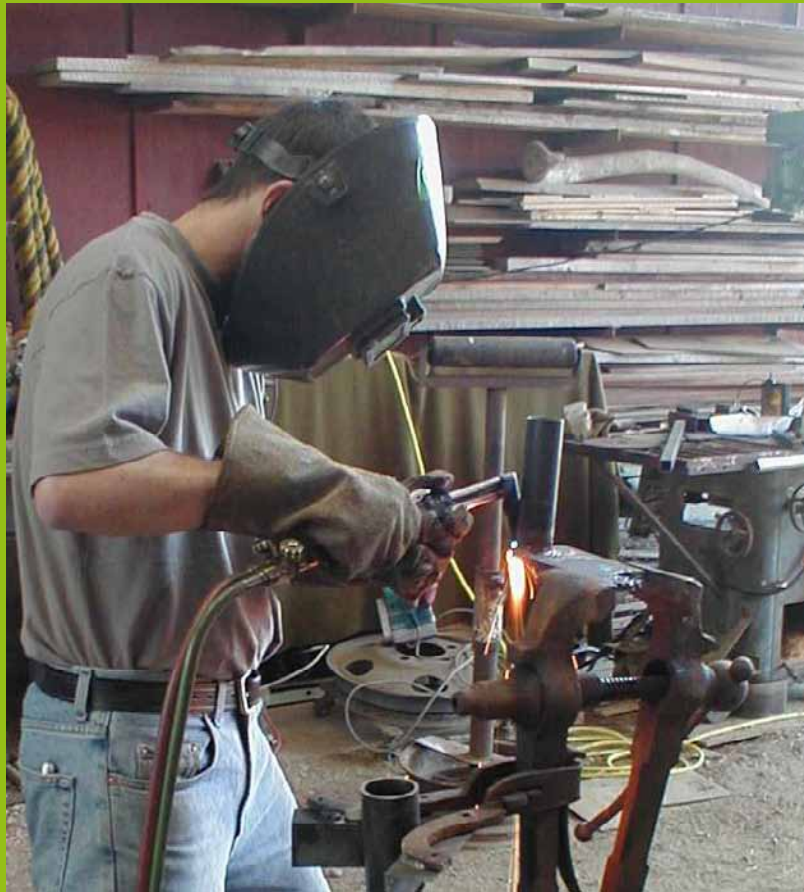
Cutting surplus plate off the top of the tail hinge outer tube.
