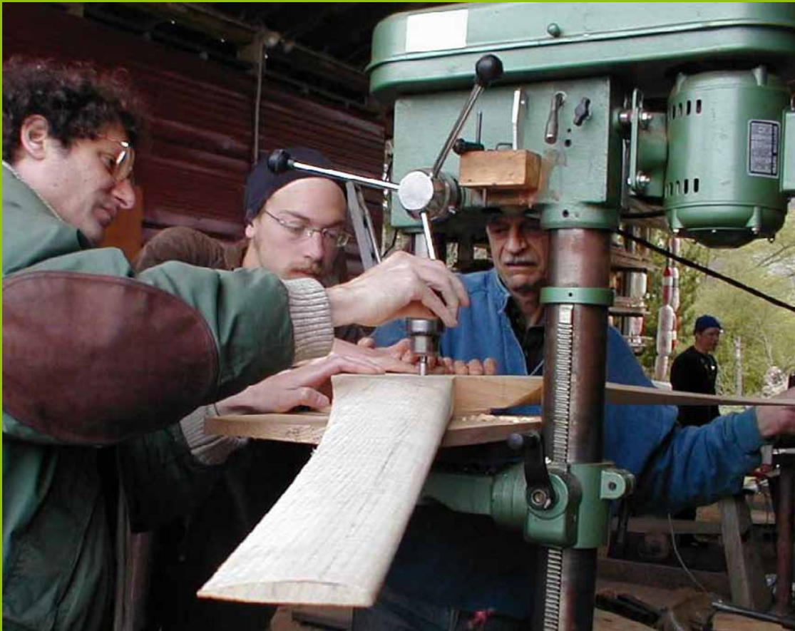
Drilling holes in the hub for mounting the blades on the front of the alternator.
