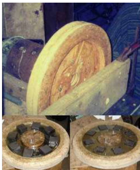
Rotor mould being made and used
