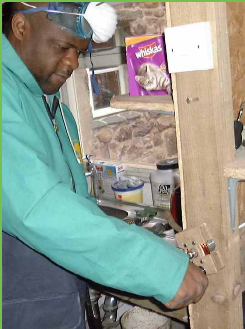
Pic 7: the hub looks like new after having been treated to a prolonged workout with an angle grinder. Unfortunately most hubs one will find at scrap yards will have worn races, with the help of inexpensive new ones our problems were solved after gently packing them with just the right amount of grease. (Here Brian is using the old bearing race, split on one side, as a drift to knock in the new one. - Hugh)
