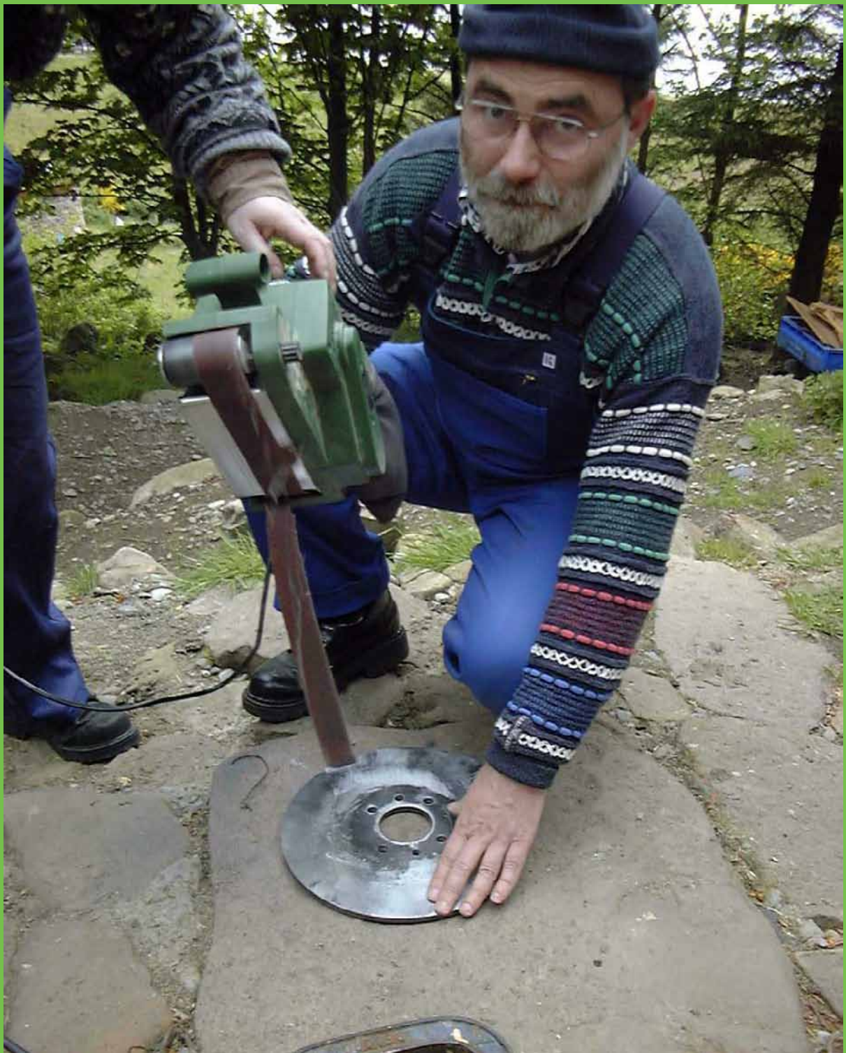
Pic 14: The metal tools were attracted by the magnets creating a force pressing the moulds together. The 2 rotor moulds are in the front, the stator mould behind. To help curing the resin we installed two heating lamps in William's winter garden. A beautiful tour of Scoraig's wind turbines was scheduled for the next day to give the resin more time to harden.
