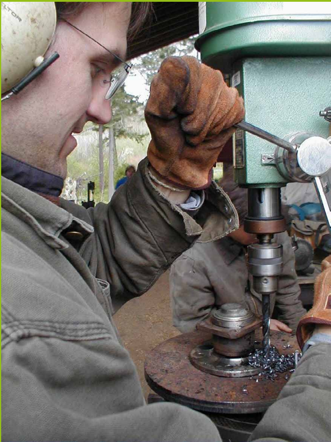
Peter drilling through the hubs and into the steel disks for perfect alignment.
