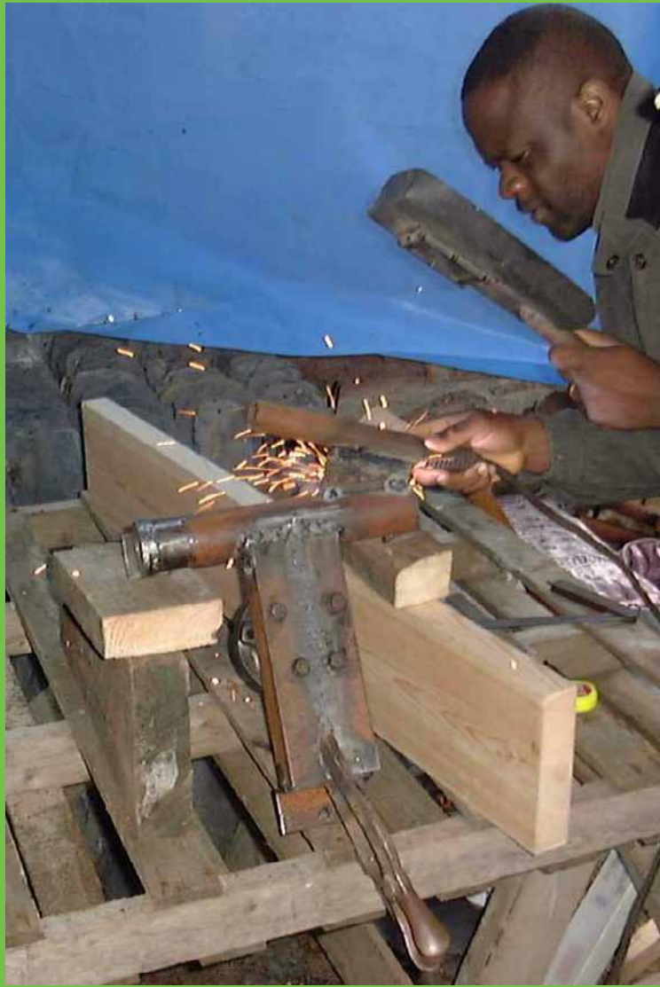
Pic 21: Here is a nice trick how to cut along 2 lines in 3 dimensions with ease, somewhat of a mind twister when trying to visualize how you are going to saw this piece while drawing it up. A hand saw really does a great job. ( These are the blade wedges - Hugh)
