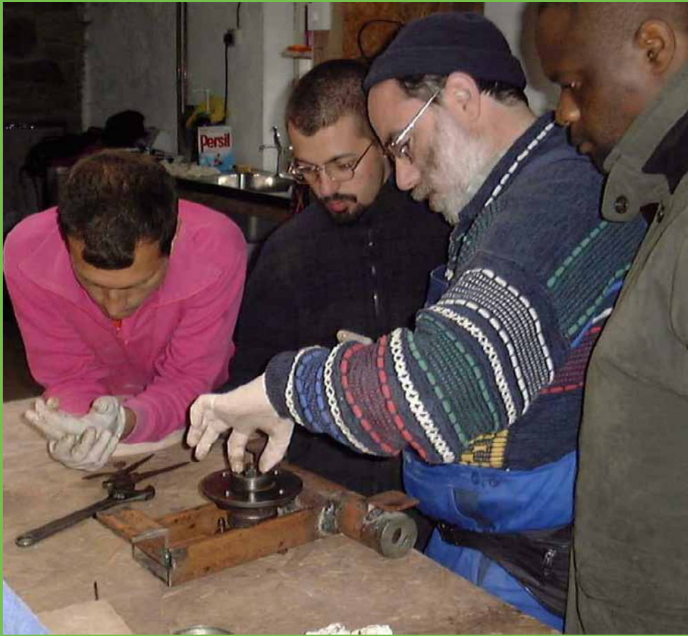
Pic 19: The wooden stator cut out comes in really handy when drilling the mounting holes. Demian and John are standing at a right angle to each other to help Uwe align the power drill vertically.
