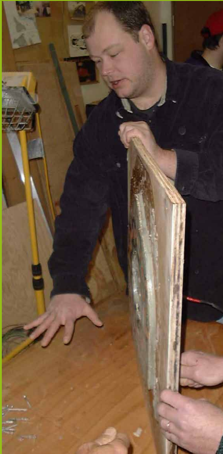
Jim VanGorden getting the stator out of the mould. The wires are holding it to the cover.
