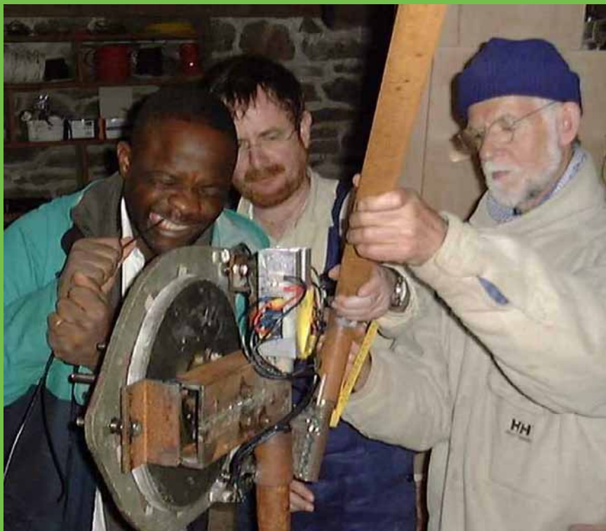
Pic 26: Lots of hands were needed to safely assemble the finished blades. It took some time to equalize the tip-to-tip distances while holding the centers together before we could clamp everything down and start drilling the mounting screw holes.
