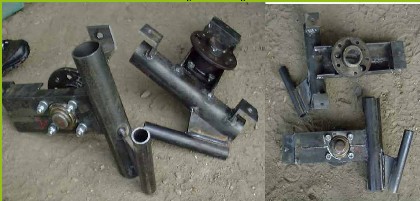
Tacking the stator lugs on.
