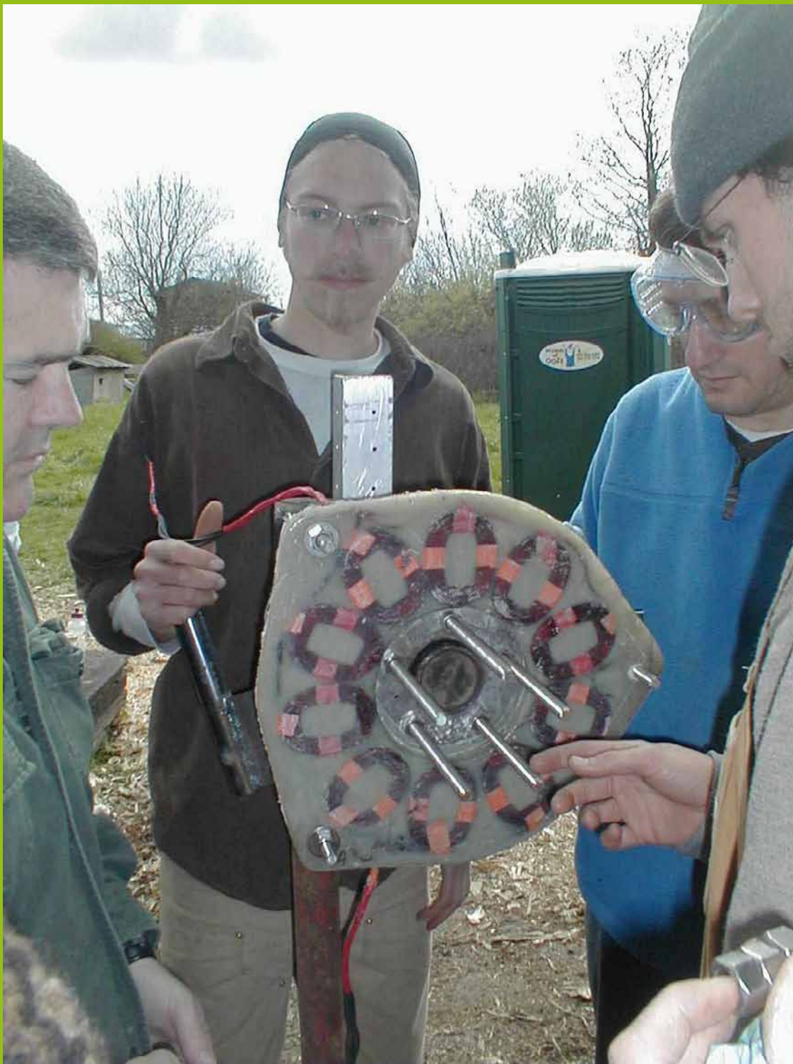
The stator on and ready for the front magnet rotor.
