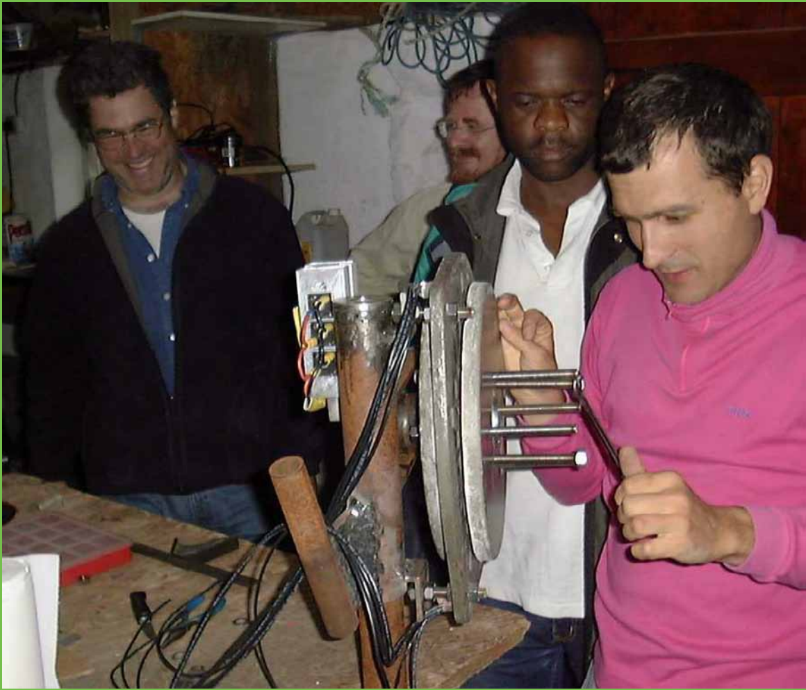
Pic 24: The diode voltage drop across the rectifier may be quite low, but even at 1 Volt and 5 to 10 Amps it starts dissipating quite some heat (5 - 10 Watts each). (Twin heat sinks for the rectifiers. - Hugh)
