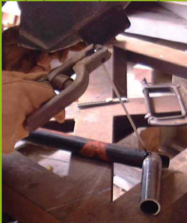
Welding the tail boom to the hinge outer pipe.
