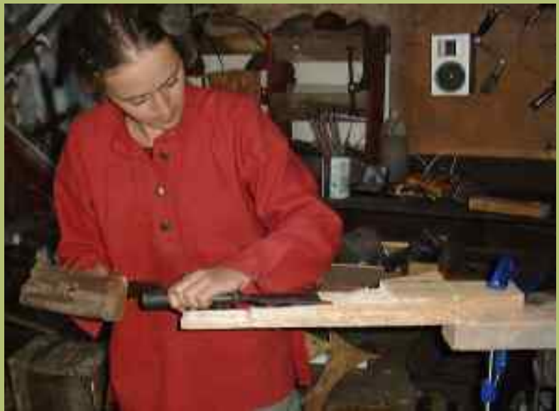
and finishing with a drawknife
