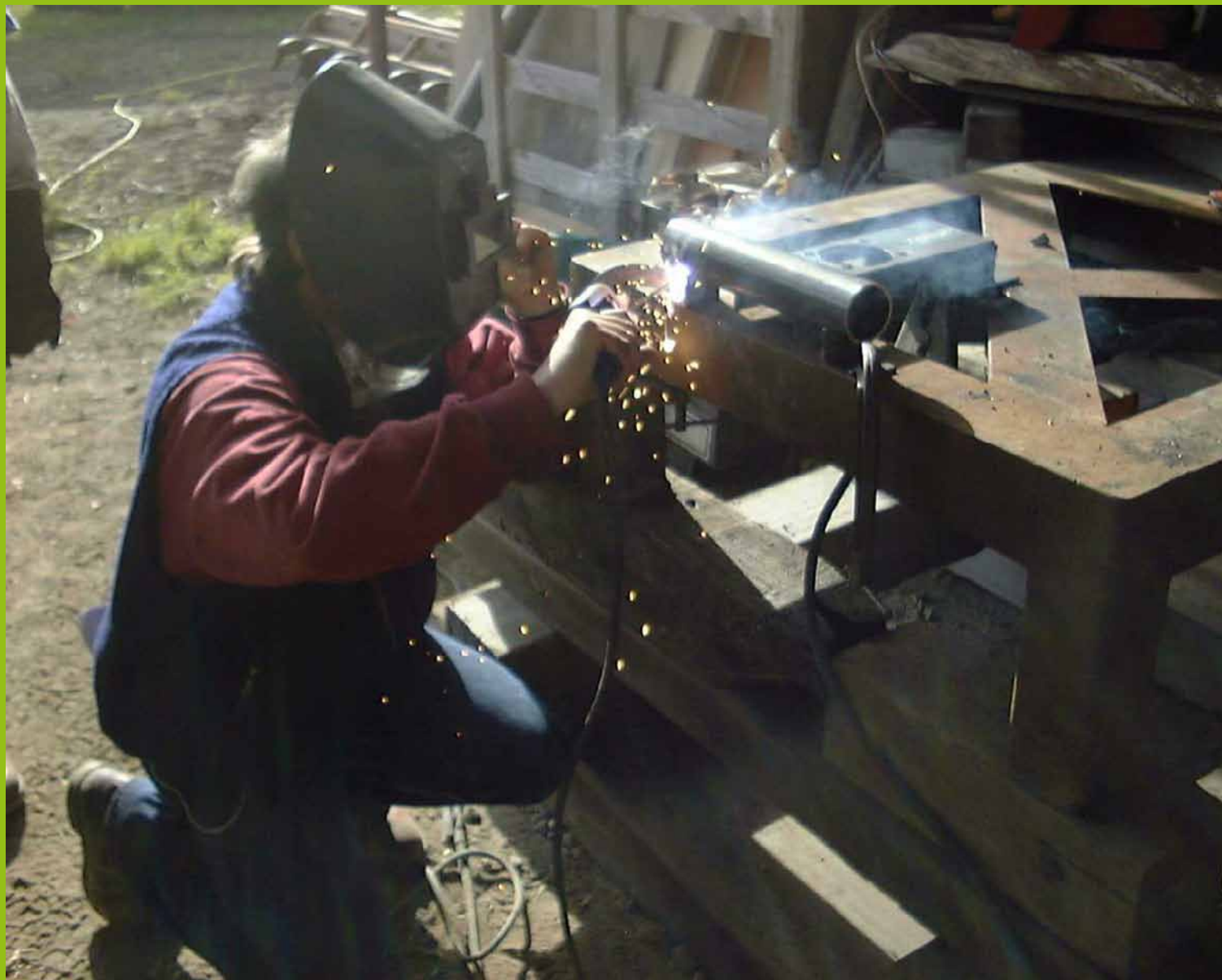
Tacking the stator lugs on.
