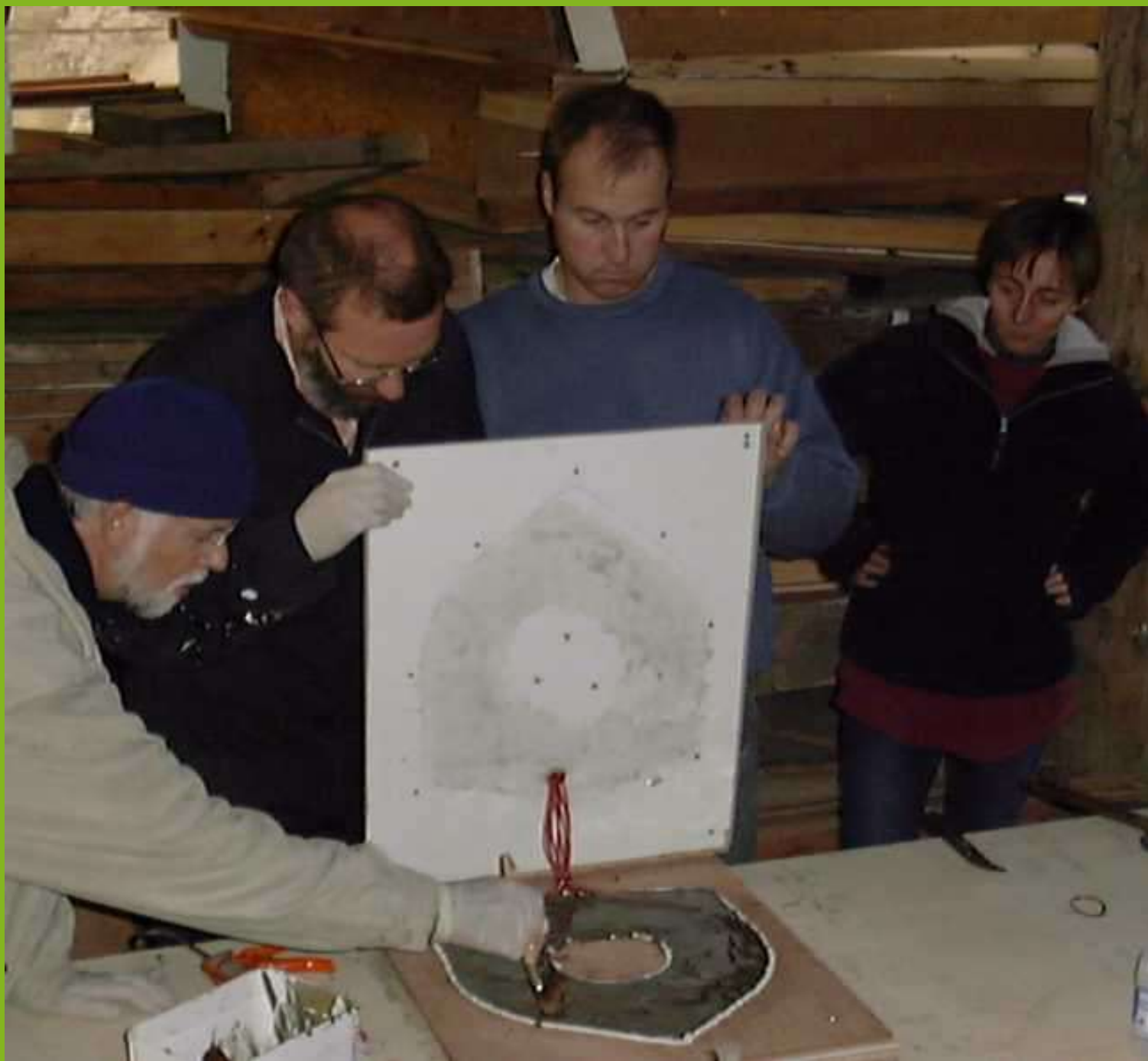
Painting the magnet disks with resin
