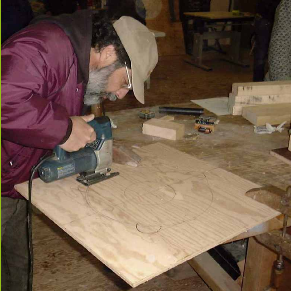
Ray cutting out a stator mould.
