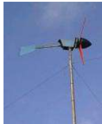
Photo 5 : Three bladed wind turbine by IT Peru. Blade diameter 1.7metres (IT Peru)
