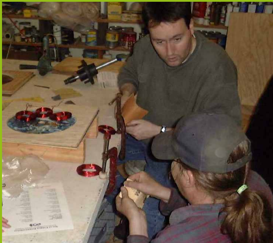
Jonathan and Dan cleaning the enamel off the wires ready for soldering.
