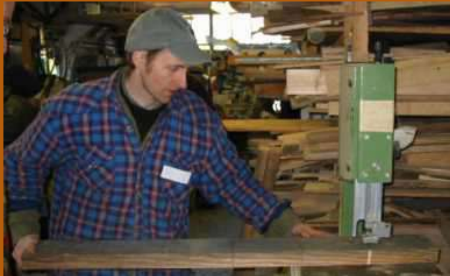
Neil cutting our the blade taper on a bands
