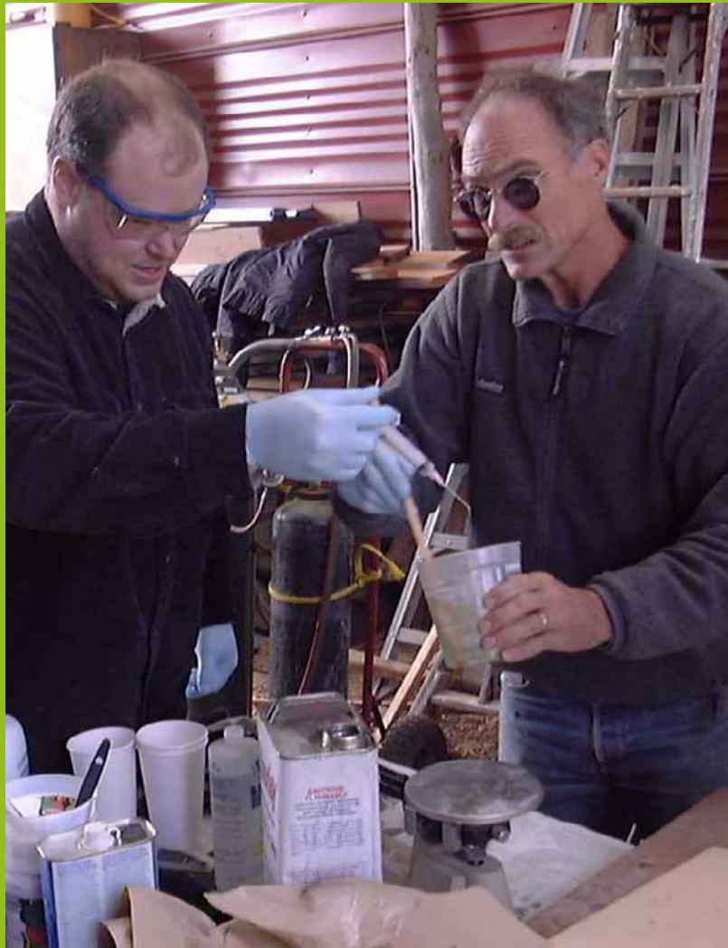
Jim and Jim mixing resin. Measuring out the catalyst with a syringe.
