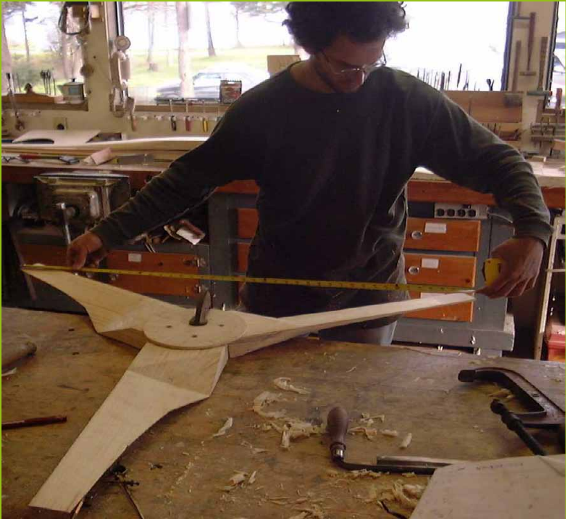
Two ways to hold the hub still while getting the tips equally spaced.
