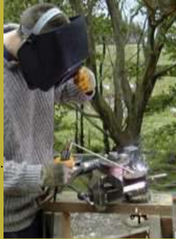
Welding the steel frame of the wind turbine.
