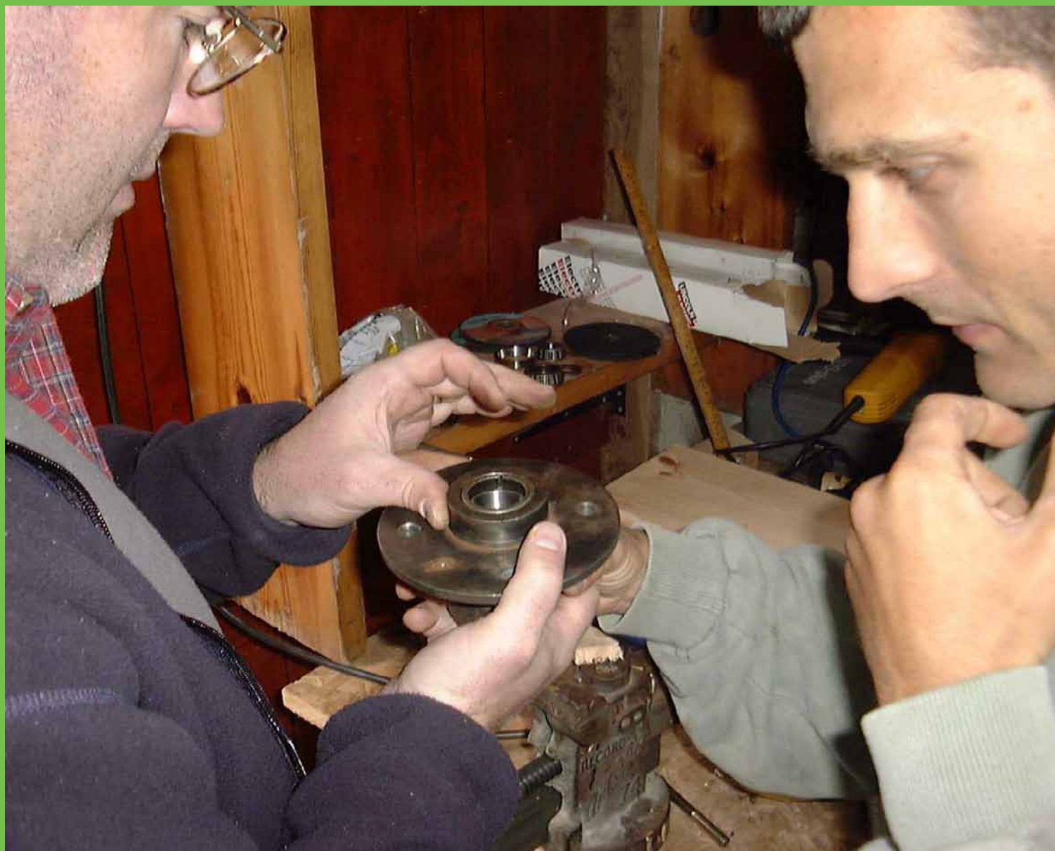
Pic 8: The beautifully laser cut extra thick steel rotor plates are drilled with the help of an often used self aligning technique. One hole is drilled through both plates and the hub for alignment (you can see the bolt holding everything in place). After aligning all three pieces, the 3 remaining holes are drilled.
