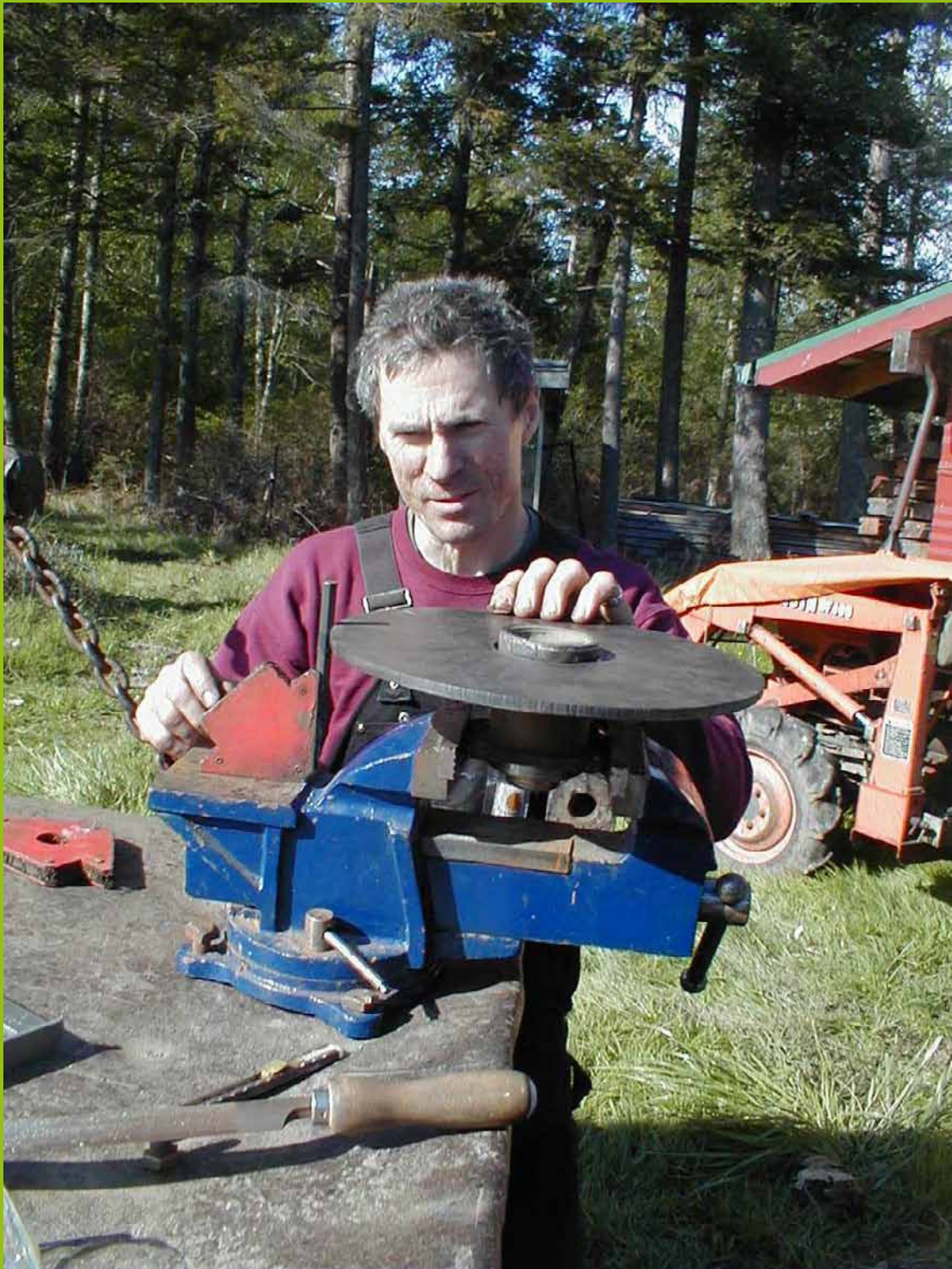
Andy getting the disks to run true before drilling.
