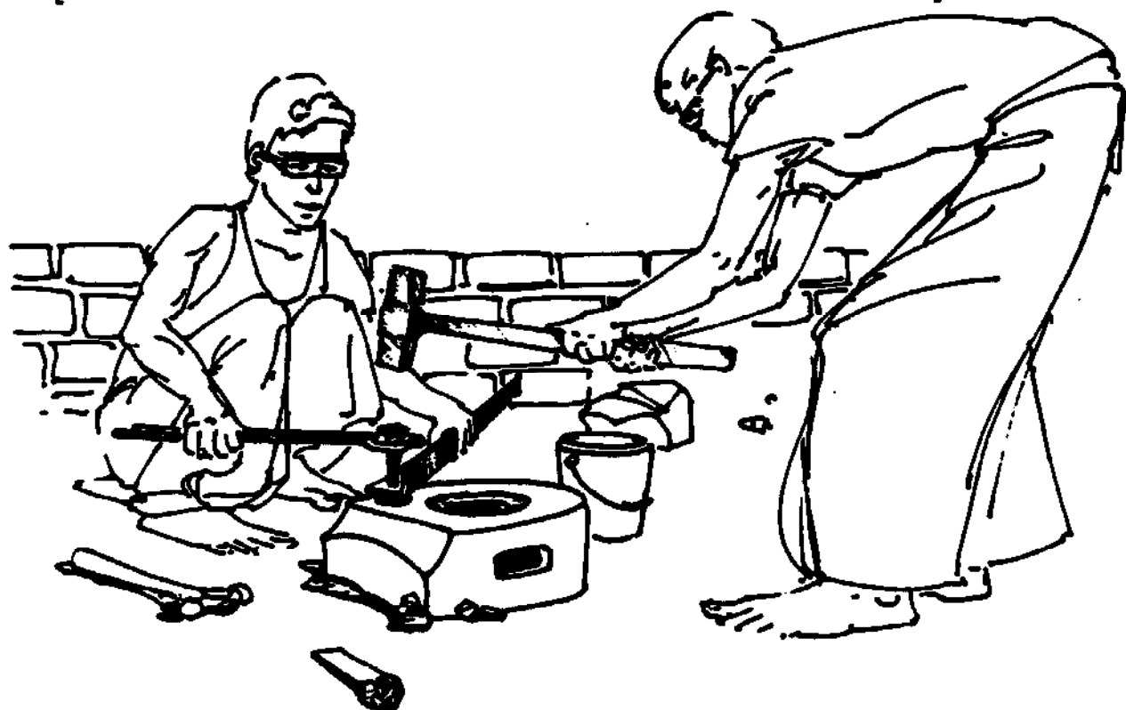
Figure 11. Using a sledgehammer, punch, and die to make a hole
