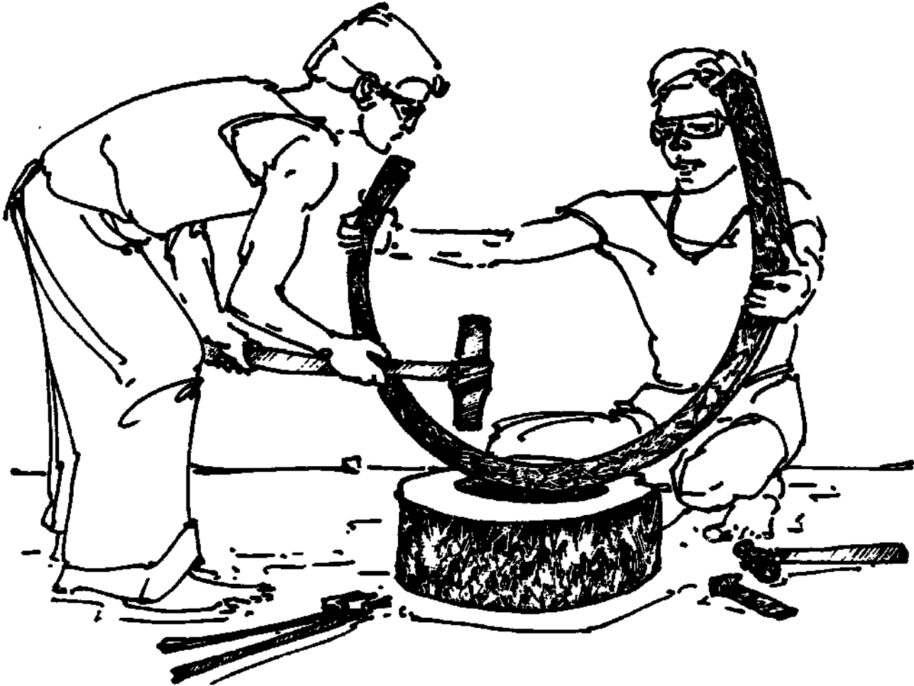
Figure 12. Bending the tower head ring
