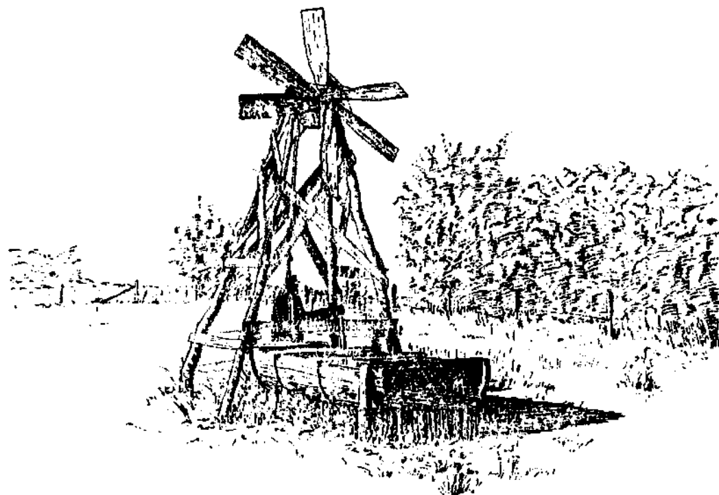
FIG. 58. The stationary six-fan Turbine mill designed and built by Frederick Mathiesen near Grand Island, giving front and side views. Made of parts from an old mower; twelve foot tower; nine foot wheel. Waters fifty head of cattle. Cost between $1 and $5.
