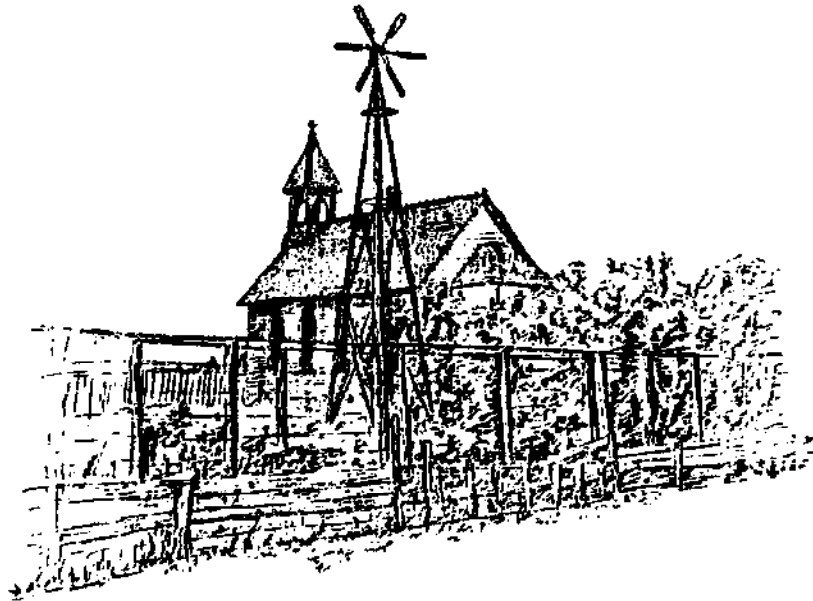
FIG. 73. The reconstructed Aermotor—a veritable toy—which cost nothing yet pumped water for the house, four head of horses, lawn, garden, and small fruit. By measurement it pumped, in a 15 \frac{1}{2} -mile wind, 270 gallons in an hour, or at the rate of 6480 gallons in twenty-four hours; that is $1 worth of water in a day according to the rate of .0015 cents a gallon, as charged in Lincoln. Wheel eight feet in diameter. Depth of well twelve feet. Property of A. C. Walker, civil engineer.
