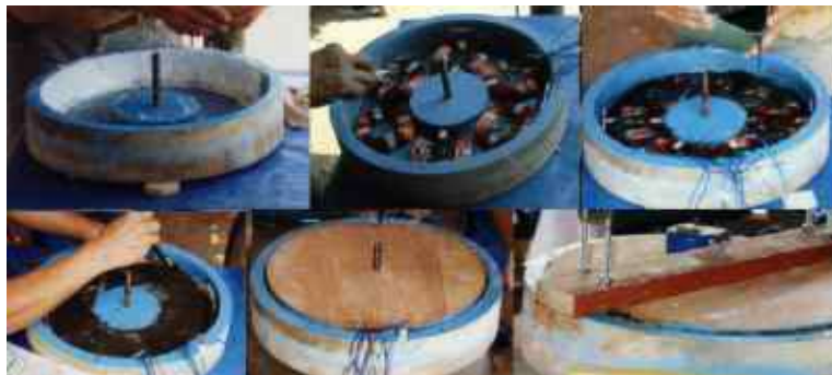
Six stages of the rotor casting procedure
