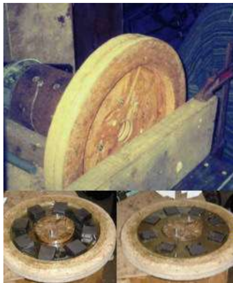
Rotor mould being made and used
