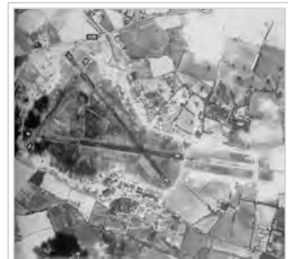
RAF Exeter airfield on 20 May 1944, showing the layout of the runways that allow aircraft to take off and land into the wind
