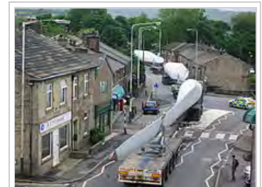
A turbine blade convoy passing through Edenfield in the U.K. (2008). Even longer two-piece blades are now manufactured, and then assembled on-site to reduce difficulties in transportation.
