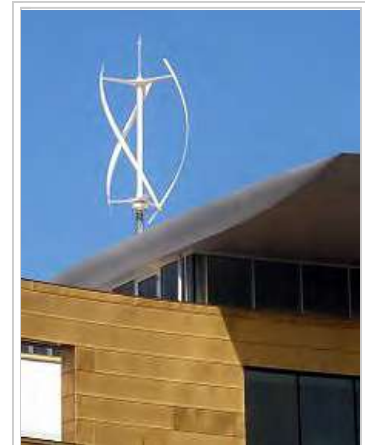
A small Quietrevolution QR5 Gorlov type vertical axis wind turbine on the roof of Colston Hall in Bristol, England. Measuring 3 m in diameter and 5 m high, it has a nameplate rating of 6.5 kW.
