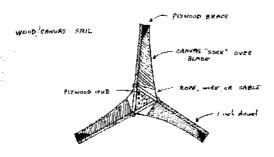
of the tower, probably at a slight dihedral angle for added stability. Higher gearing will be necessary (about 20:1), but we feel that a larger blade diameter (15 feet), simple construction, and less centrifugal stress will make the test worthwhile.
