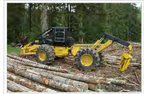
Modern dual function grapple skidder
