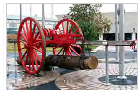
A slip tongue log skidder used in the 19th and early 20th centuries.
