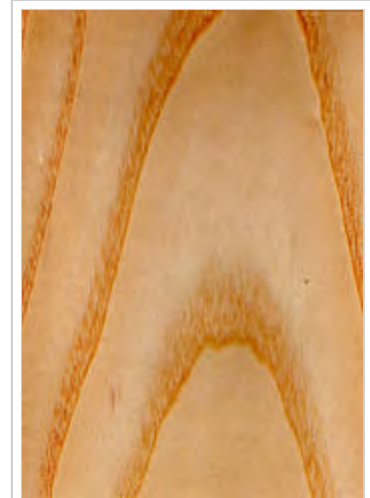
Earlywood and latewood in a ring-porous wood (ash) in a Fraxinus excelsior ; tangential view, wide growth rings
