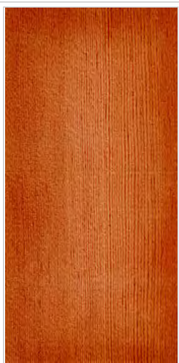
Earlywood and latewood in a softwood; radial view, growth rings closely spaced in Rocky Mountain Douglas-fir
