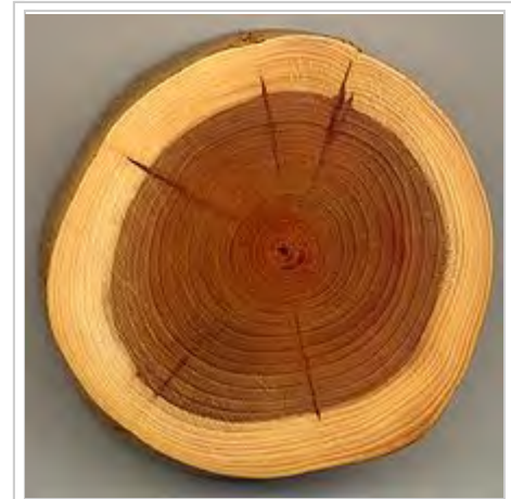
A section of a Yew branch showing 27 annual growth rings, pale sapwood, dark heartwood, and pith (center dark spot). The dark radial lines are small knots.
