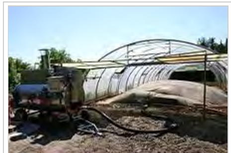
Sheet steaming with a MSD/moeschle steam boiler (left side)
