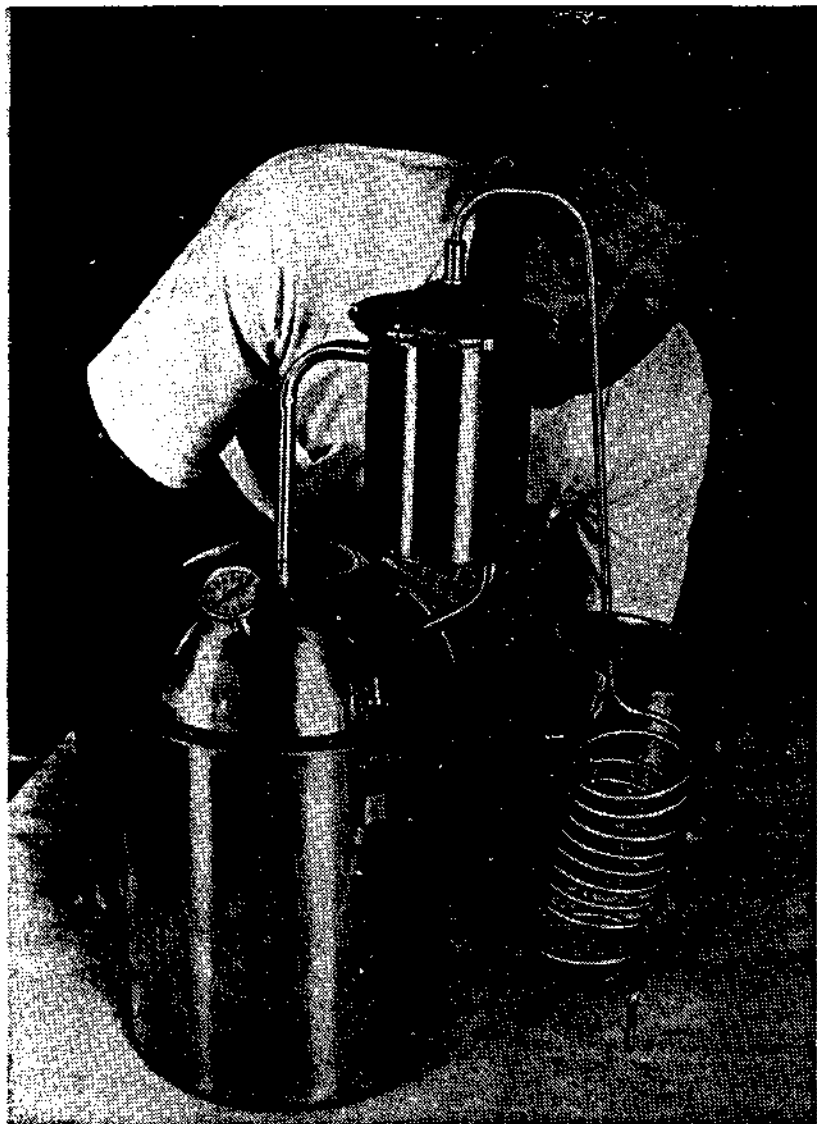
Fig. 10-1. Tabletop still capable of producing enough fuel for a lawnmower or moped.
