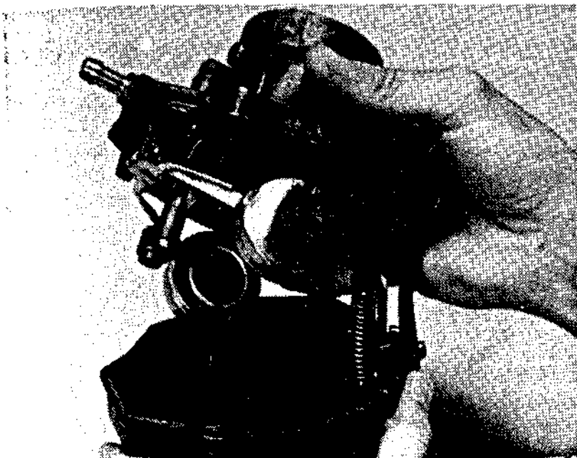
Fig. 13-1. To burn straight alcohol fuel, the carburetor must be modified to produce a richer air/fuel mixture. This involves partially disassembling the carburetor to change the main fuel metering jet (courtesy Mother Earth News).
