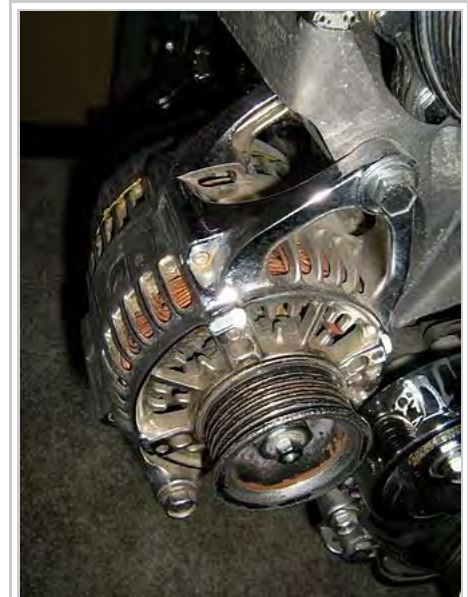
Alternator mounted on an automobile engine with a serpentine belt pulley
