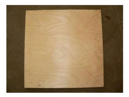
Start by cutting out an 18" square piece of plywood. This will be the bottom of the mold
