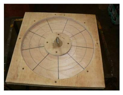
Put a bit of epoxy on the threads of the threaded rod. You may need to double nut the end of the threaded rod but usually you can screw it in by hand. Screw the threaded rod into the hole so that the bottom of the rod comes flush with the bottom of the mold. If any epoxy comes up to the top of the mold wipe it off with a rag.
