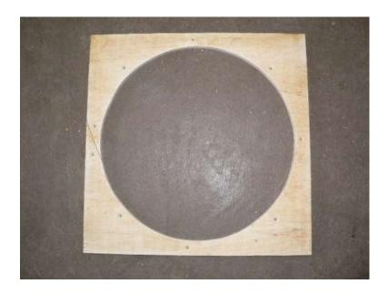
Make another plywood square just like the last one (18" square) and cutout a hole in the center 15.5" in diameter. This is the middle of the mold. Sand the cuts on the inside smooth and try
