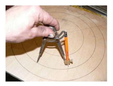
Use dial calipers to adjust your compass as shown in the picture. Then pick a starting point on the 12" circle and use the compass to divide the circle into 9 equal parts. This is a nice way to divide any circle - it's very handy for placing magnets and coils accurately in different sized wind turbines.
