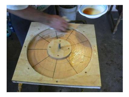
Wipe the mold down with boiled linseed oil. This will help fill the pours in the wood. When we grease the mold before casting, this assures that the grease will not soak into the mold and the castings will come out more easily. It also protects the mold from water.
