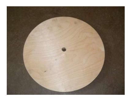
Cut out another disk from birch plywood, 16" diameter. This is the lid for the mold. Sand the edges smooth. Drill a 3/4" diameter hole in the center and give it a slight taper with a round file. (sand paper wrapped around a wooden dowel or bolt works nicely too)
