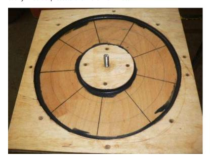
Once the linseed oil is dry run a bead of caulk around the edges of the inside of the mold. This will help create a 'tapered' mold, it will also plug any cracks between pieces of plywood to help assure the castings come out easily.
