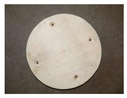
Cut out another disk 5.75" in diameter. This will be the island in the center of the mold. It also needs to be sanded smooth and slightly tapered. Drill 4 holes for wood screws as shown in the picture
