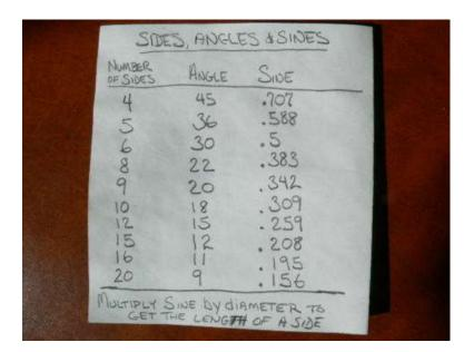
The table of sides, angles and sines for the most common numbers we use in these alternators. The angle given is half the actual angle of any segment. To use the table, pick the number of segments (sides) you need to
