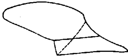
Fig. 4-9. Plow bottom showing area, below dotted line, which receives 75 percent of the draft when plowing, illustrating the necessity of keeping shares sharp for light draft of the plow.
