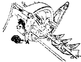
Fig. 4-61. Eccentric A is adjusted to left to take up lag in cutter bar.
