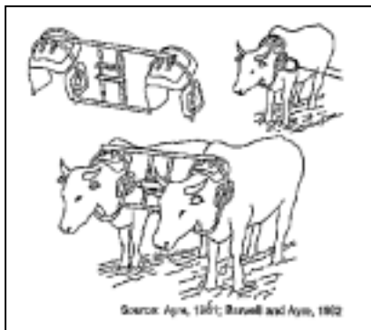
Fig.4-11: These prototype "Allahabad" single and double harnesses performed well in some research studies, but they were not adopted by farmers. Source: Ayre, 1981; Barwell and Ayre, 1982
