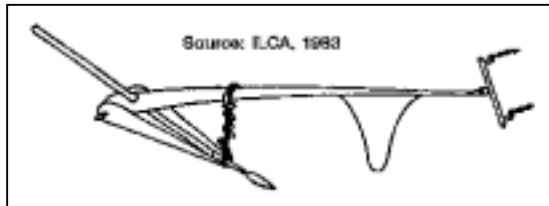
Fig 7-8: A modified malesha arc. It was developed in Ethiopia by the International Livestock Centre for Africa (ILCA) to allow use by a single animal. The beam was shortened and a skid and swingle tree were fitted. On-station trials were encouraging, but farmer uptake has been low. Source: ILCA, 1983
