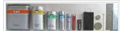
4.5-Volt, D, C, AA, AAA, AAAA, A23, 9-Volt, CR2032 and LR44 cells.
